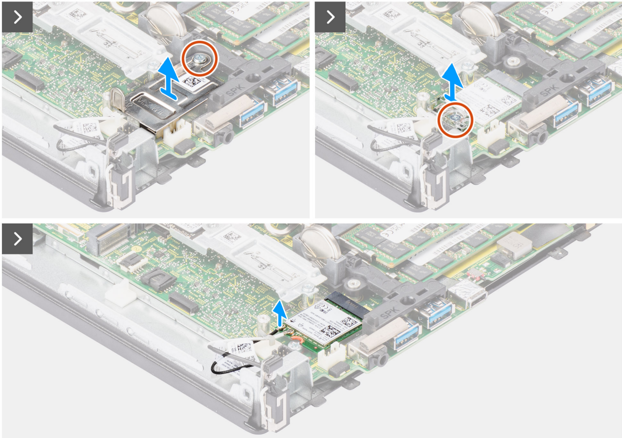
Figure 54. Removing the internal antenna—location 2
