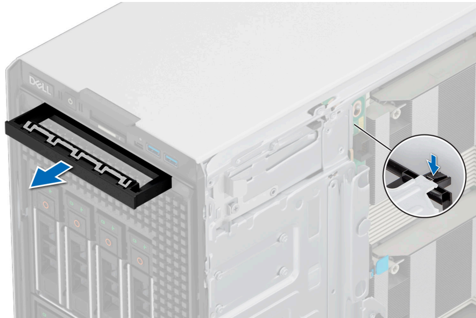
Figure 125. Removing the optical drive blank
