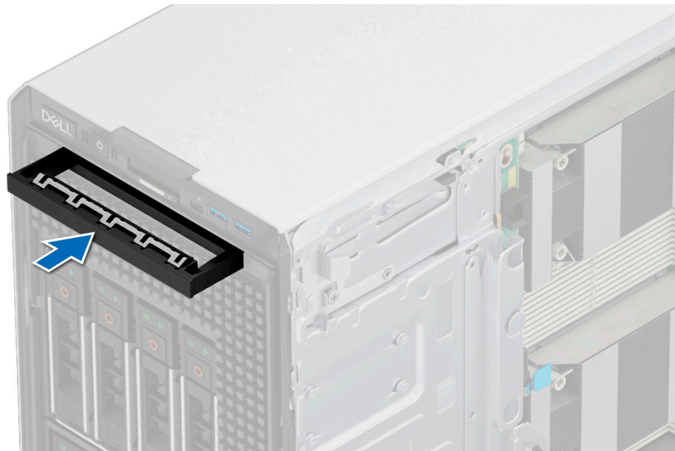
Figure 126. Installing the optical drive blank
