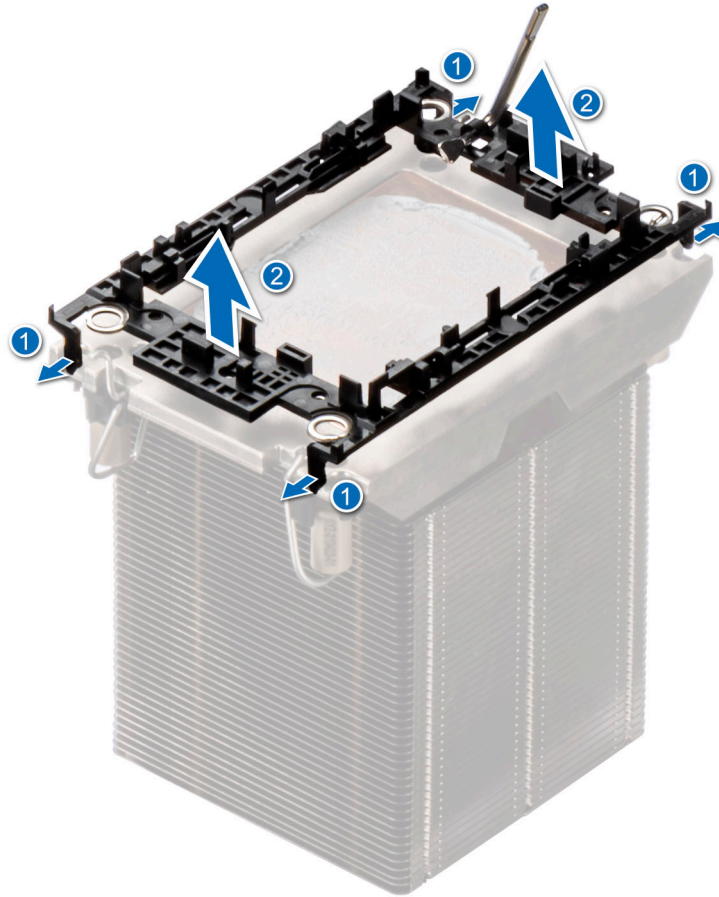
Figure 164. Removing the retaining clip
