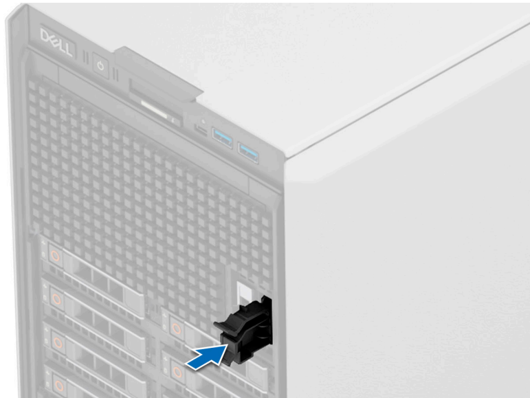
Figure 144. Installing the BOSS-N1 card carrier blank
