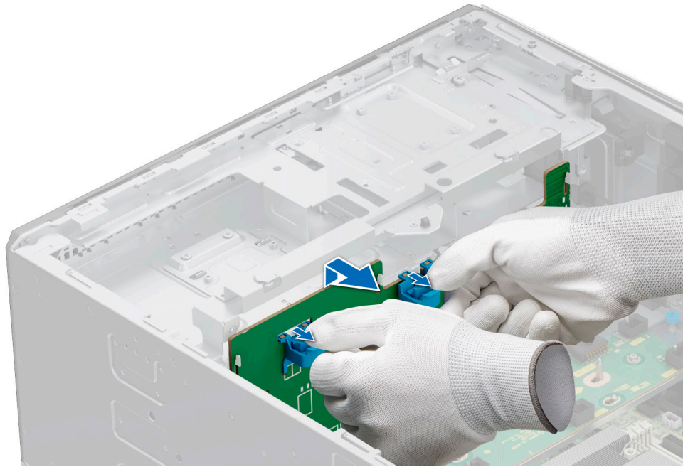
Figure 109. Removing the 3.5-inch drive backplane
