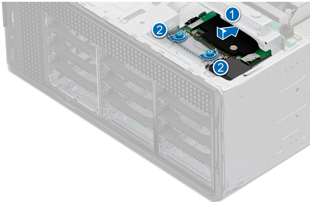
Figure 98. Installing the front PERC module to the 3.5-inch drive backplane
