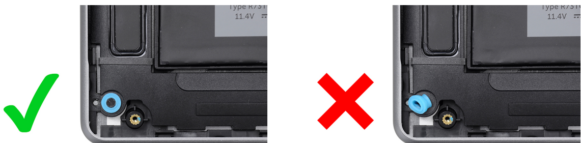
Figure 24. Installation of rubber grommets
