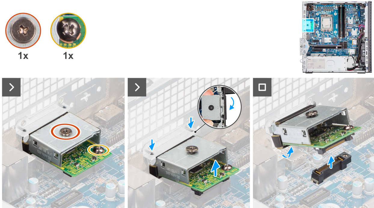
Figure 76. Removing the optional DisplayPort module
