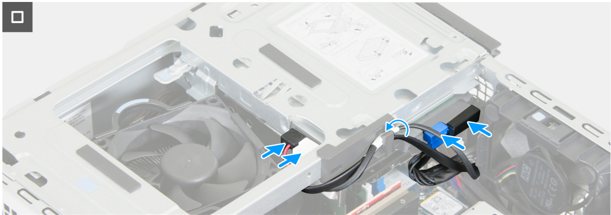
Figure 24. Installing the drive bay
