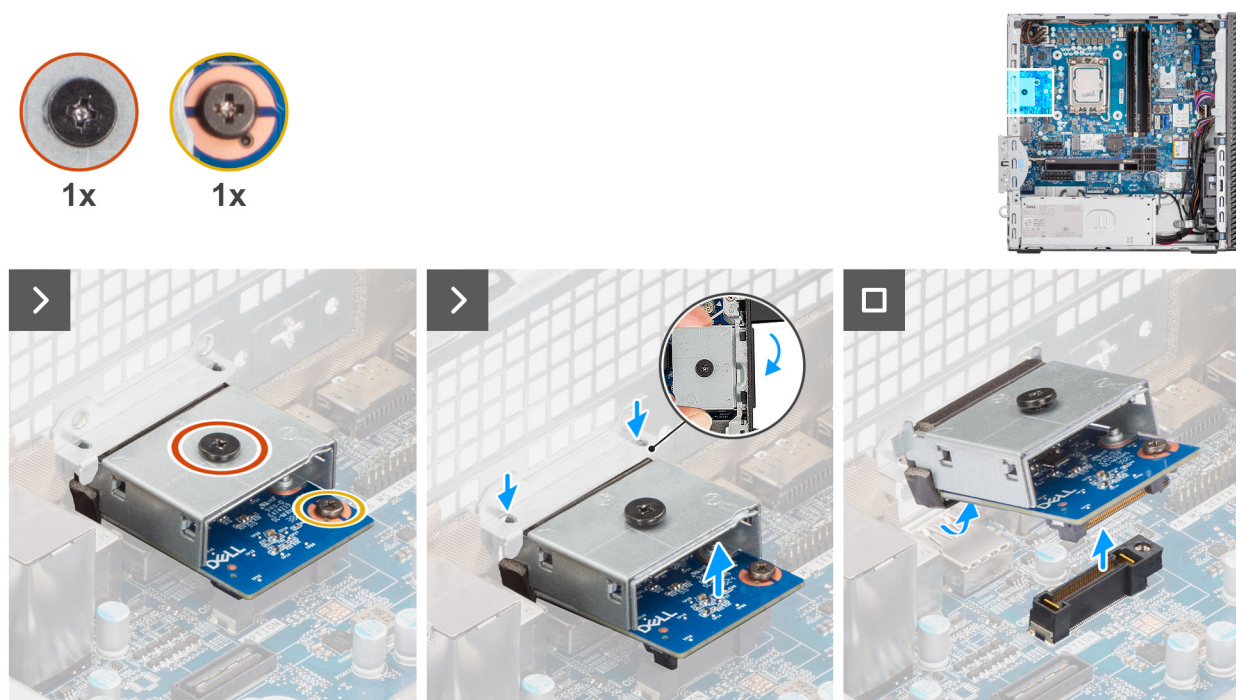
Figure 61. Removing the optional VGA module
