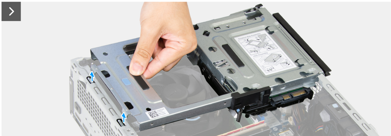
Figure 21. Removing the drive bay
