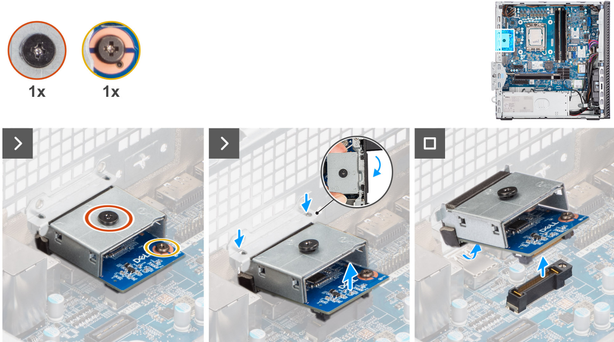
Figure 73. Removing the optional HDMI module
