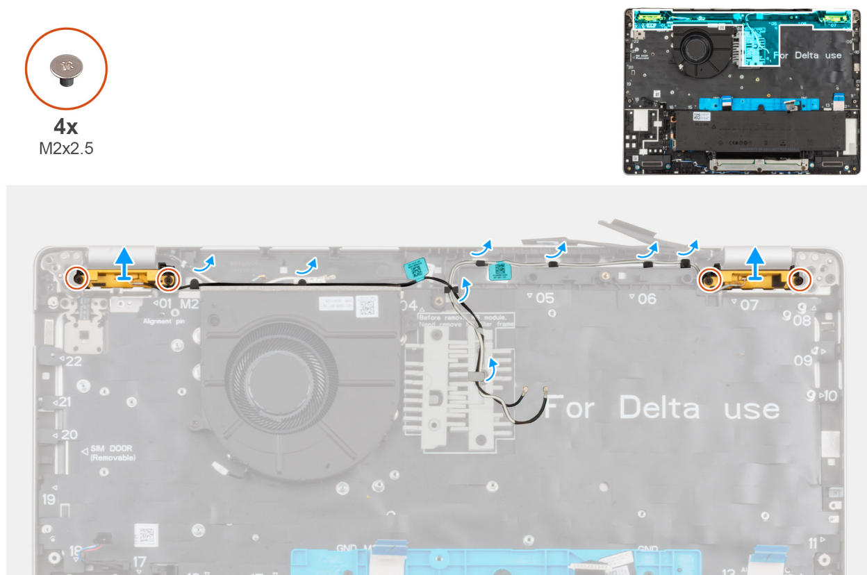
Figure 78. Removing the WLAN antenna module
