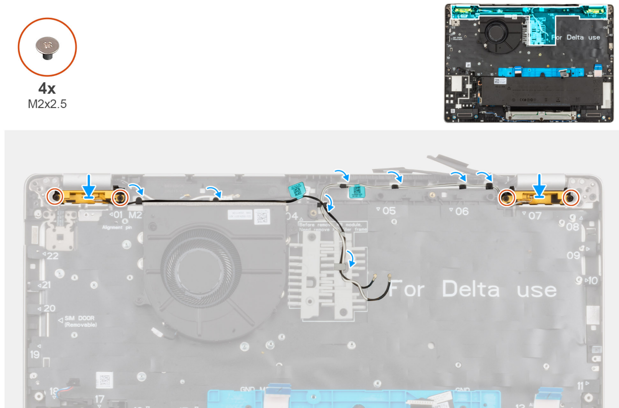
Figure 79. Installing the wireless antenna
