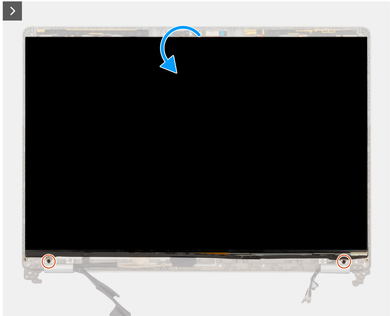
Figure 58. Removing the display panel
