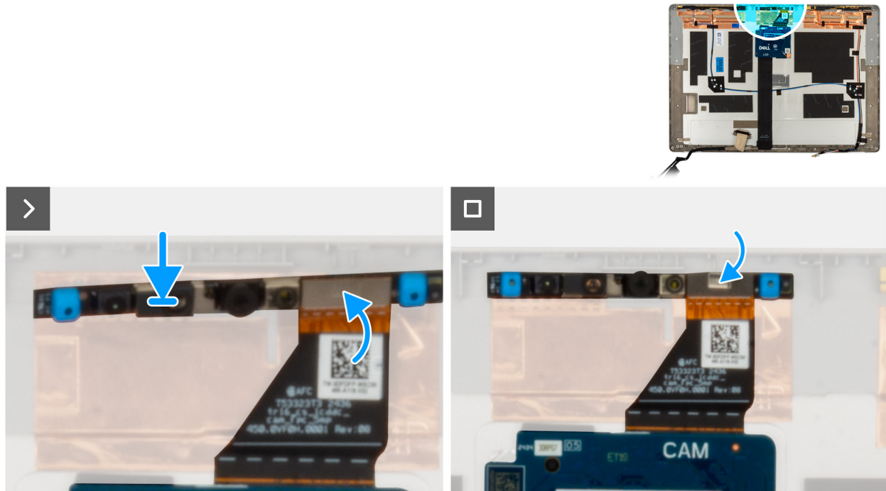
Figure 75. Installing the camera module
