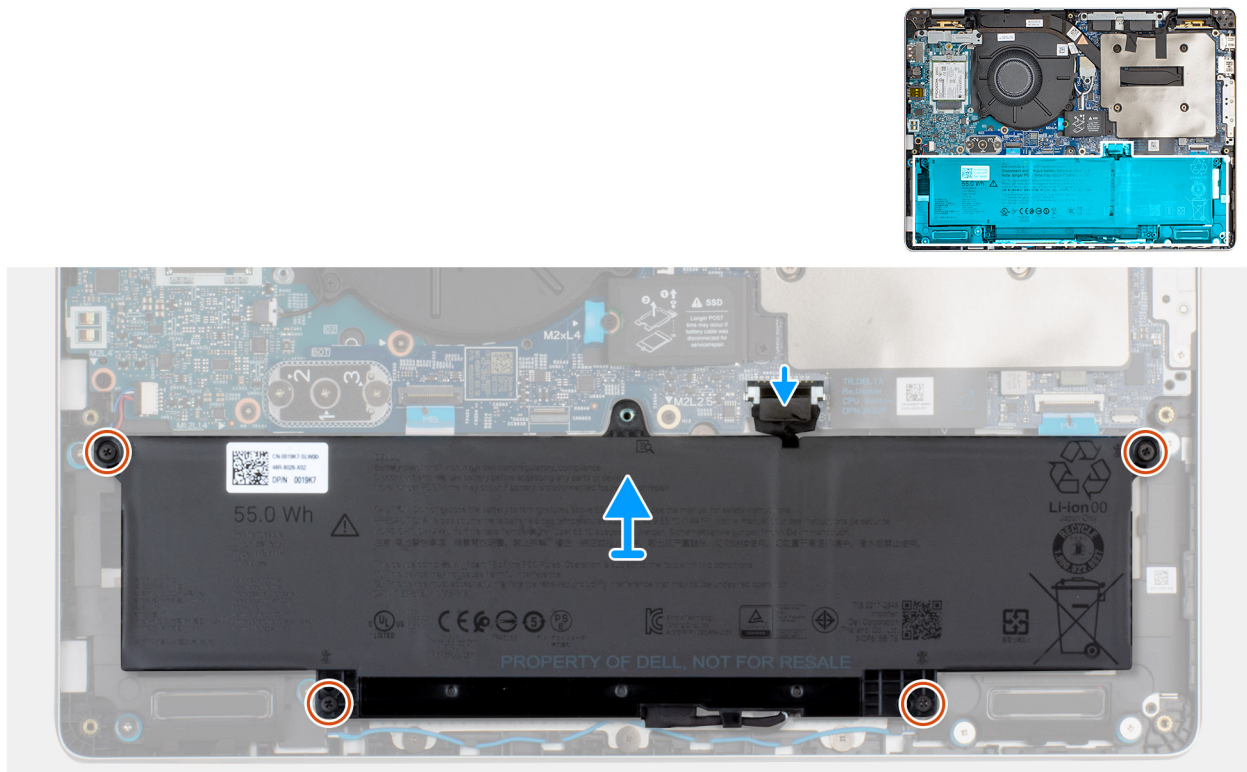
Figure 16. Connecting the battery cable
