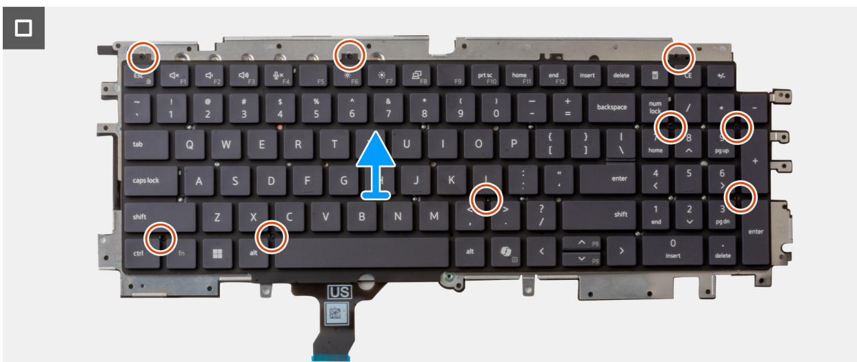
Figure 81. Removing the keyboard
