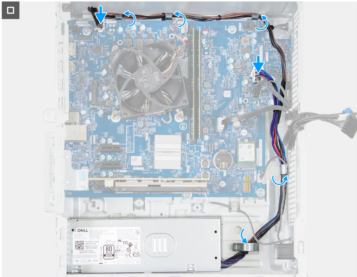
Figure 66. Installing the power-supply unit
