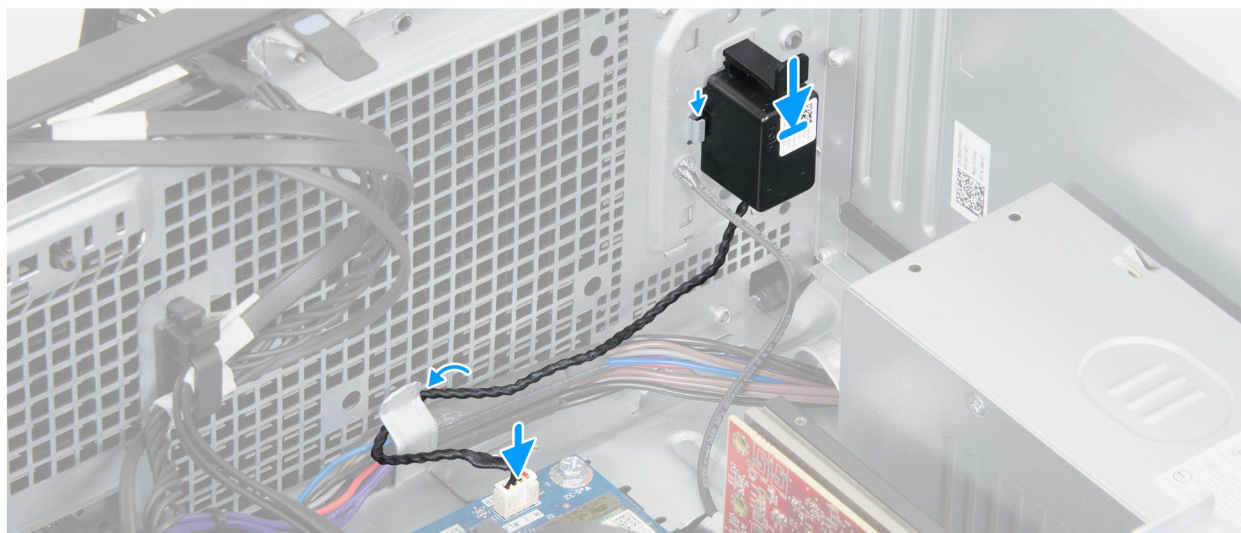
Figure 26. Installing the internal speaker
