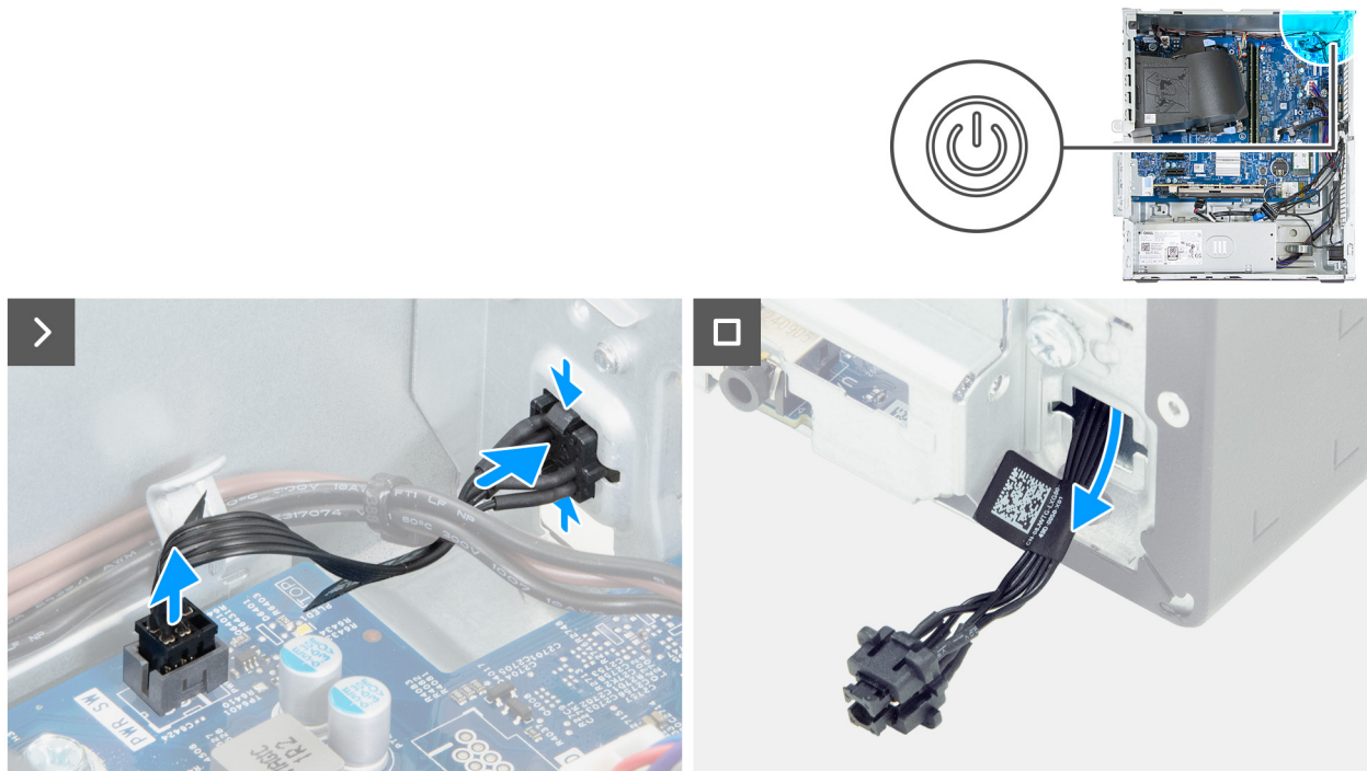
Figure 51. Removing the power button
