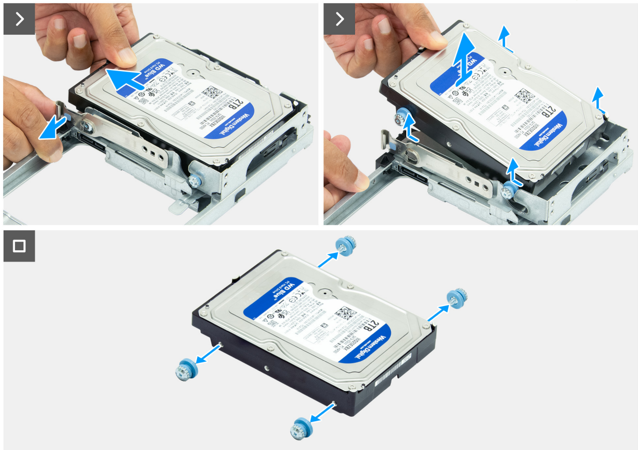
Figure 47. Removing the hard drive
