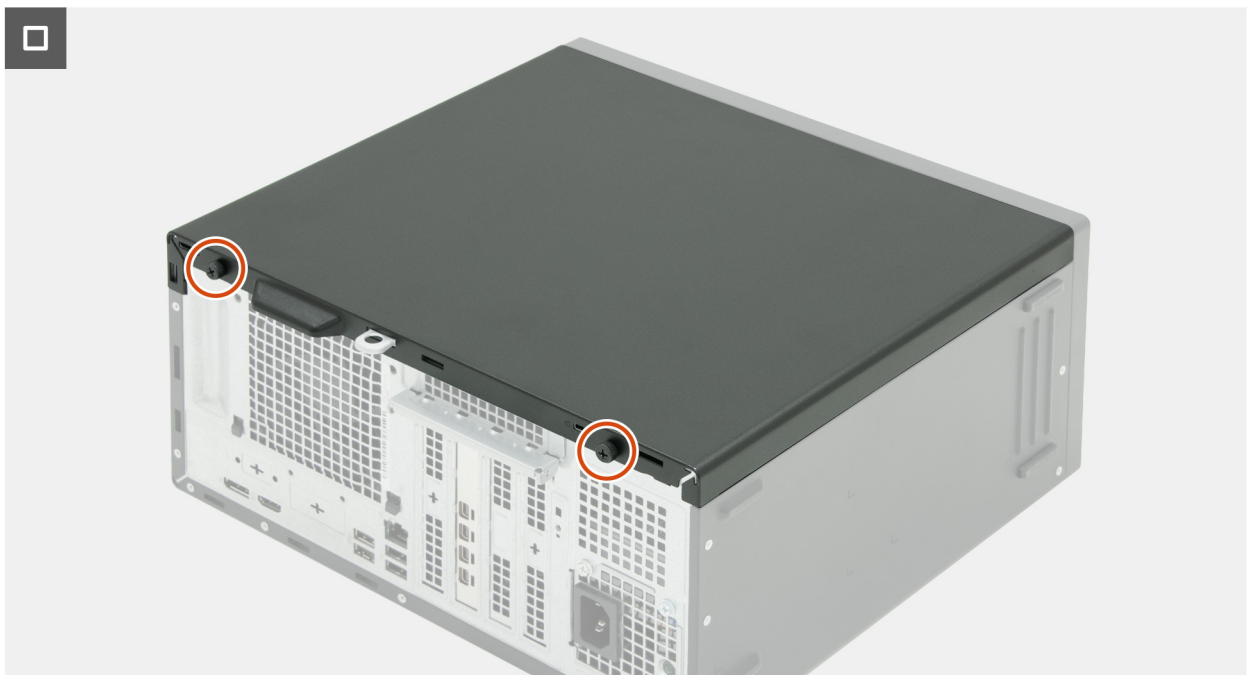
Figure 16. Installing the left-side cover
