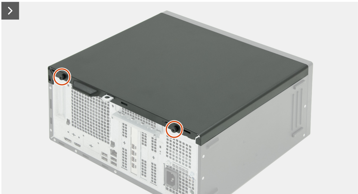
Figure 13. Removing the left-side cover
