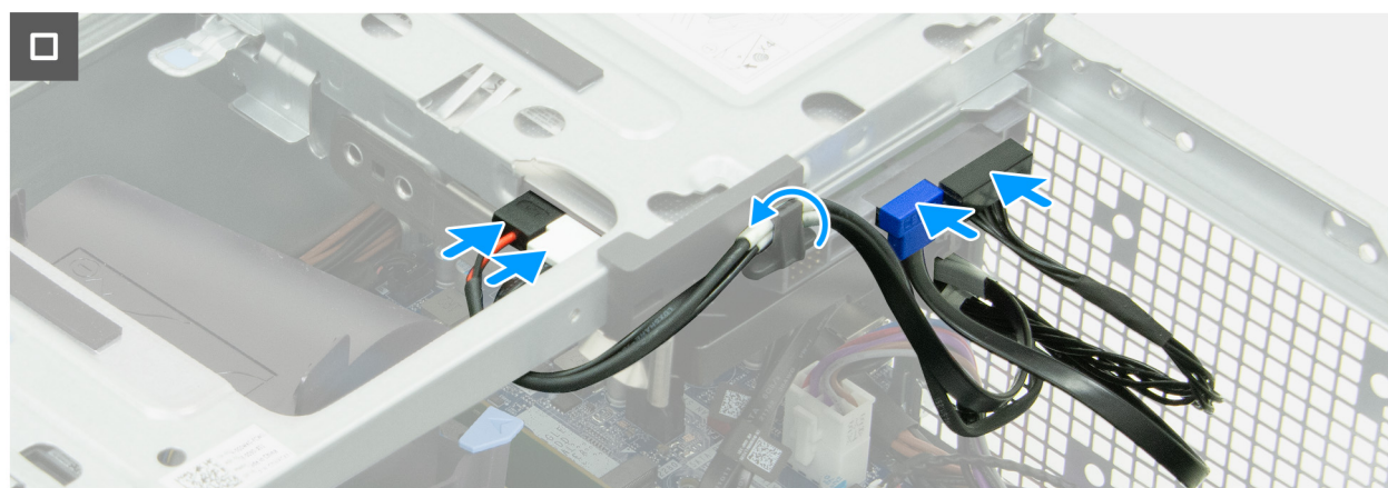
Figure 46. Installing the drive bay
