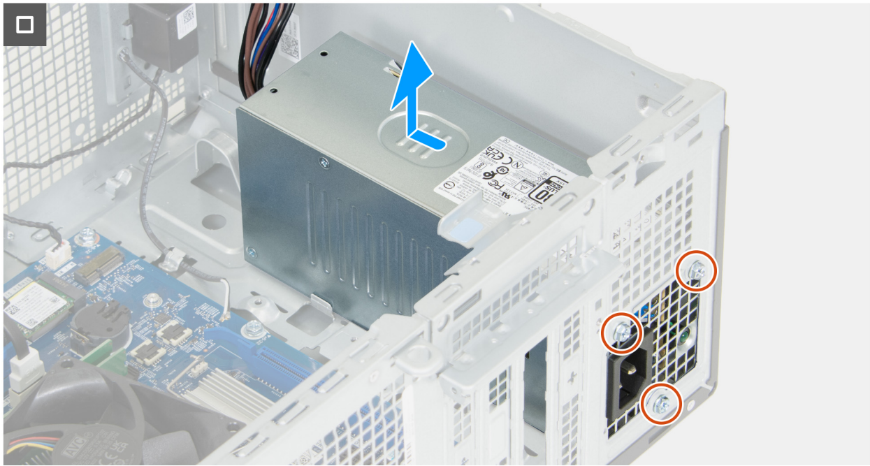
Figure 64. Removing the power-supply unit
