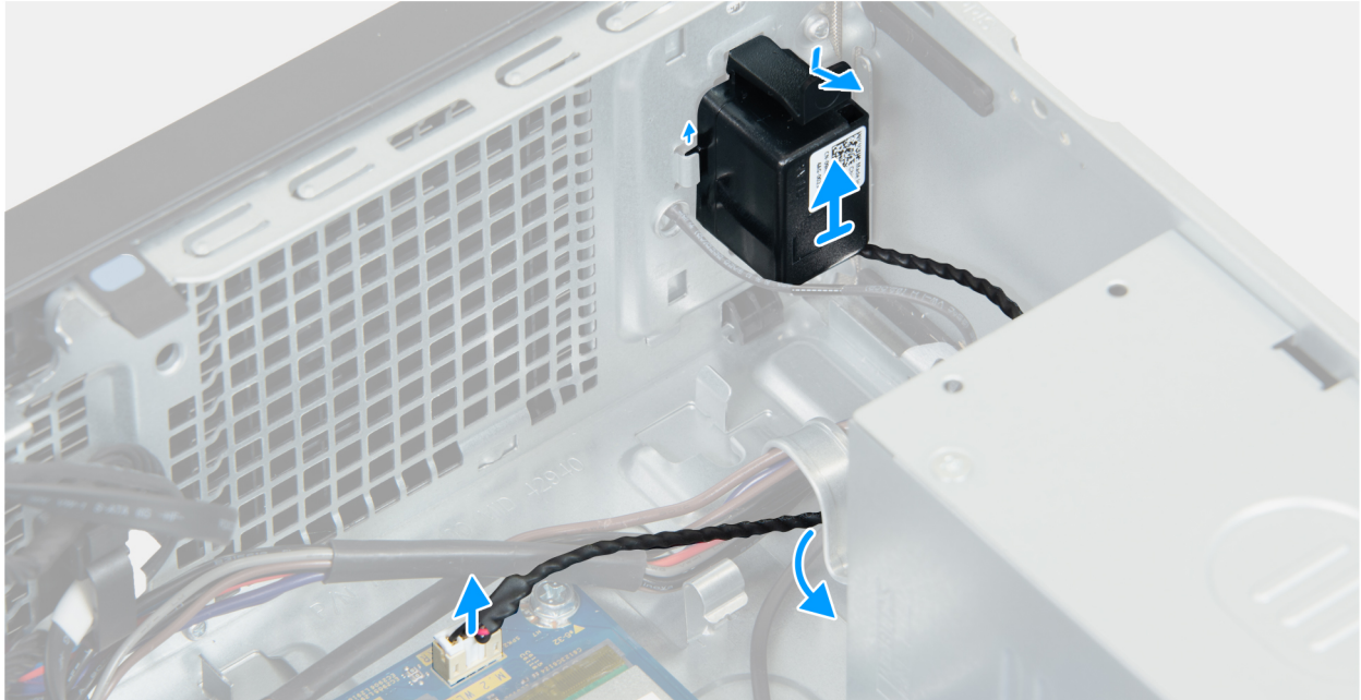
Figure 18. Removing the internal speaker
