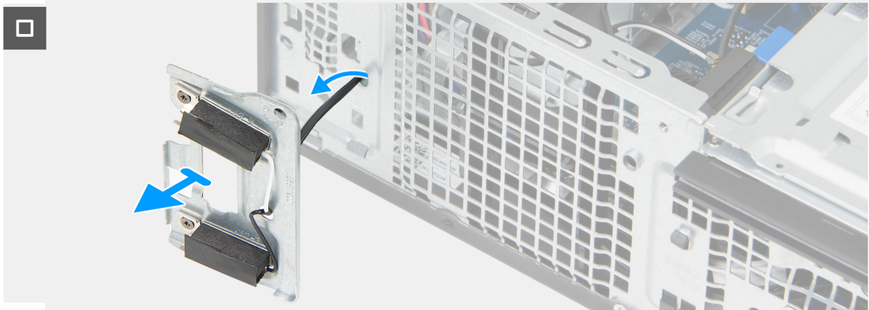
Figure 46. Removing the antenna modules
