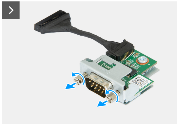
Figure 58. Installing the serial-port module
