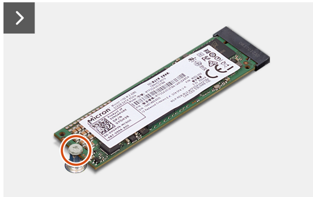
Figure 24. Removing the M.2 2280 solid state drive
