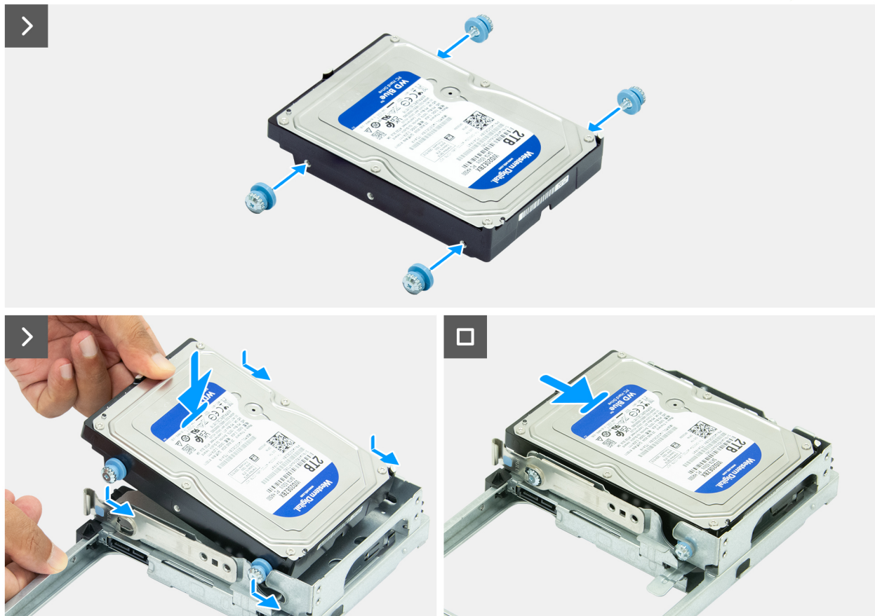
Figure 41. Installing the hard drive
