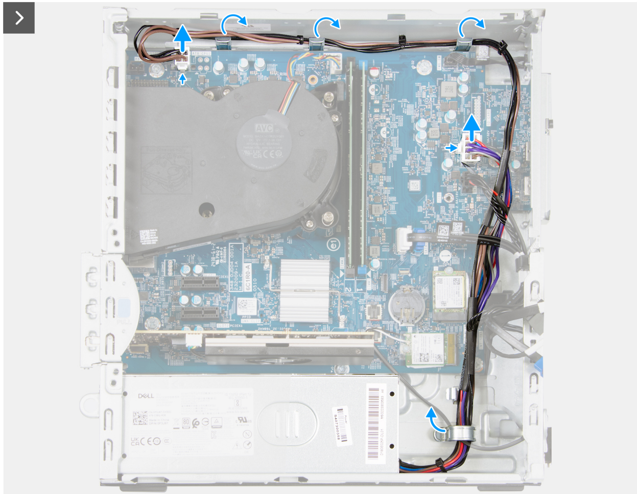
Figure 48. Removing the power-supply unit
