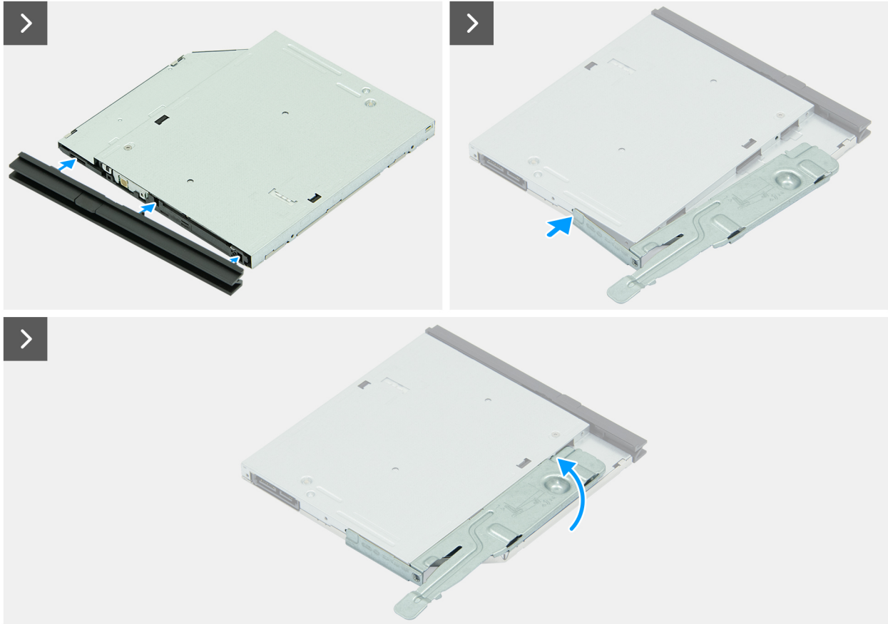
Figure 33. Installing the optical drive
