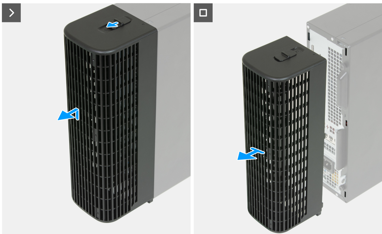
Figure 4. Removing the cable cover
