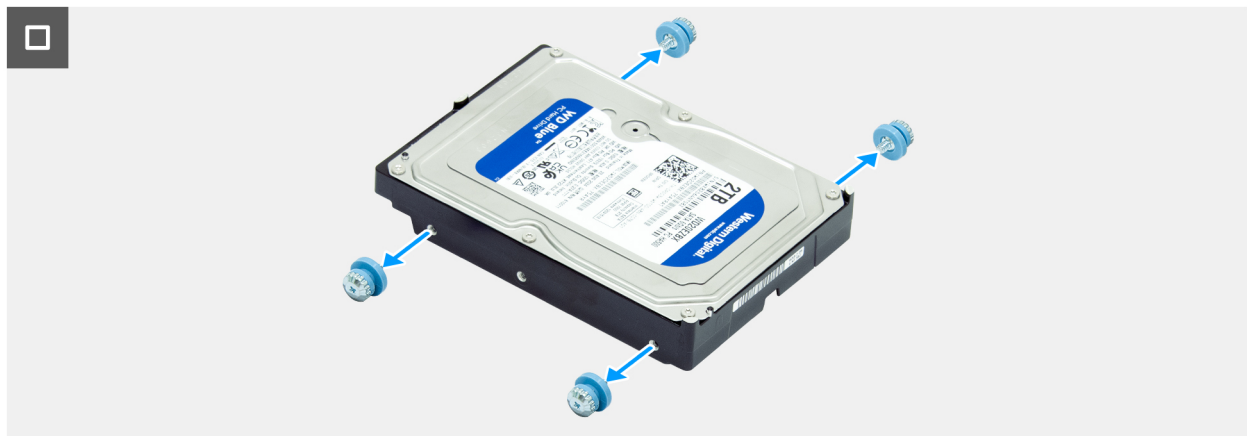
Figure 40. Removing the hard drive
