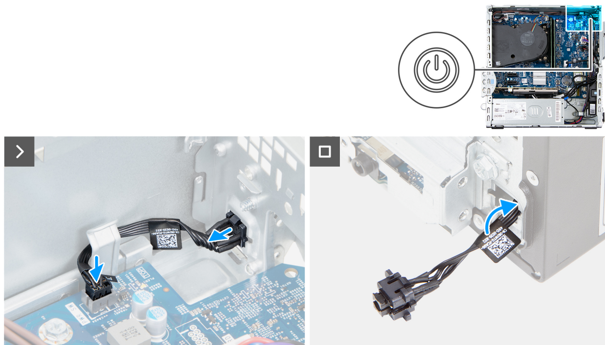
Figure 45. Installing the power button
