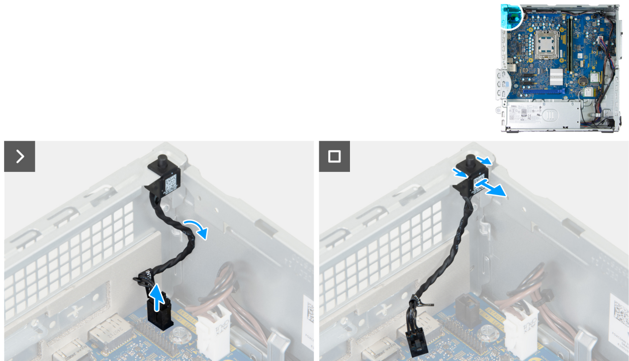
Figure 42. Removing the intrusion switch
