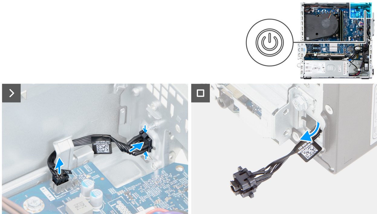
Figure 44. Removing the power button
