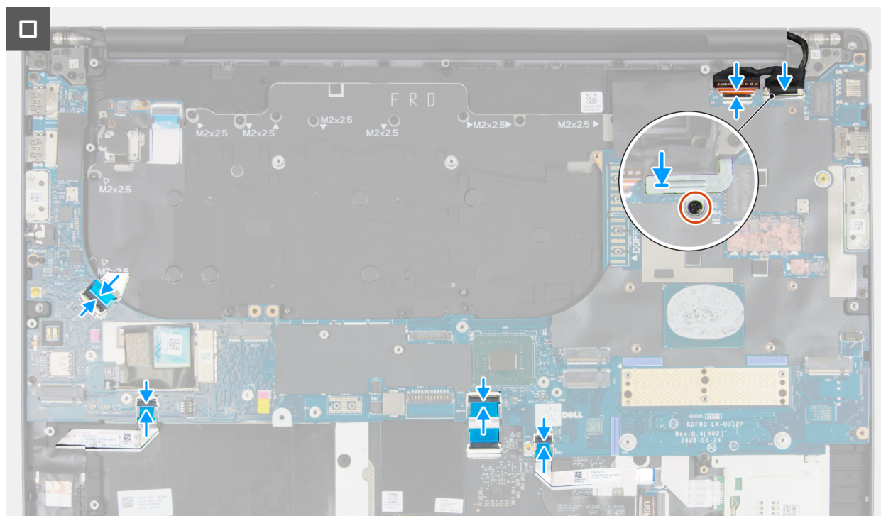
Figure 112. Installing the system board
