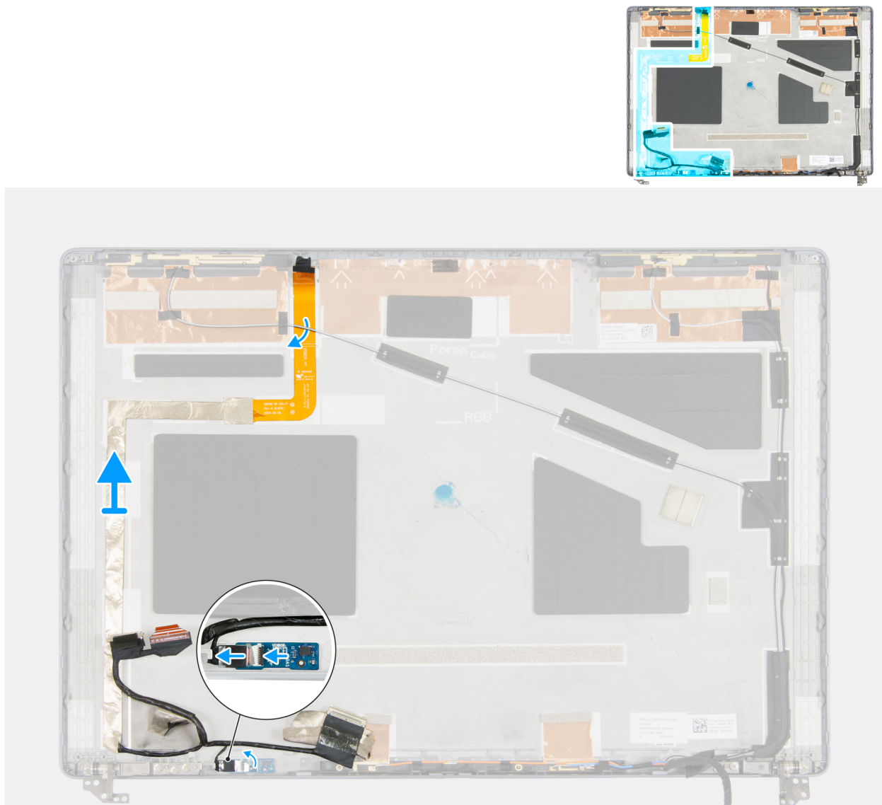
Figure 102. Removing the display cable
