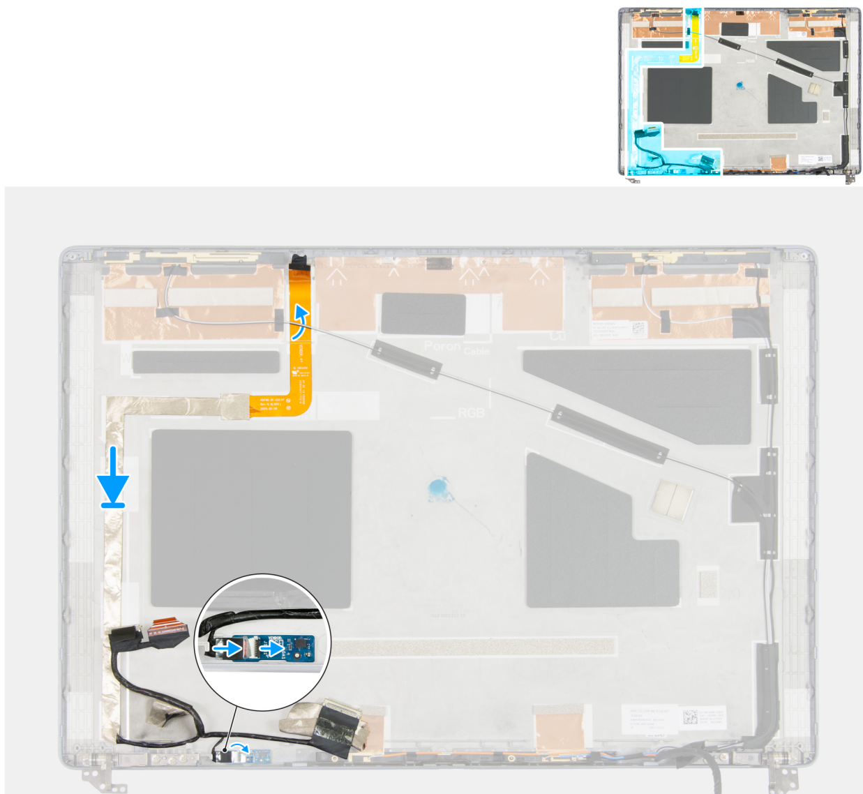
Figure 103. Installing the display cable
