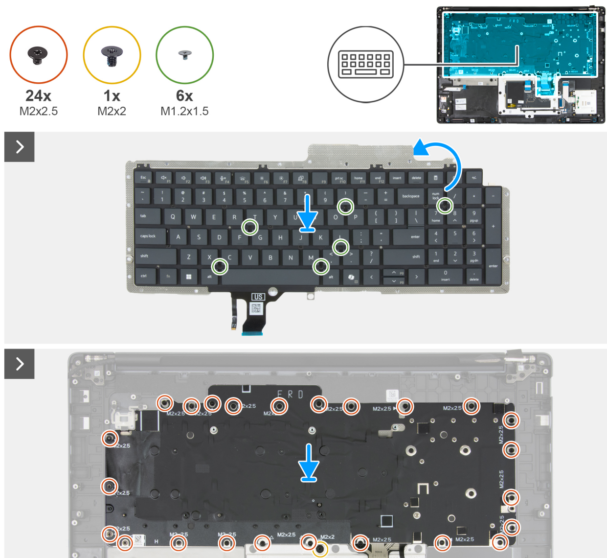
Figure 119. Installing the keyboard
