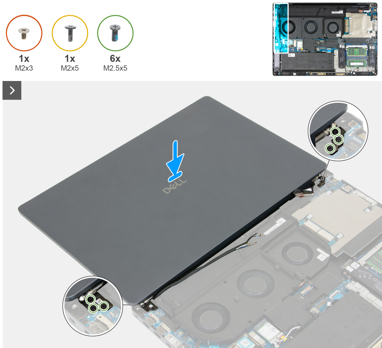
Figure 65. Installing the display assembly
