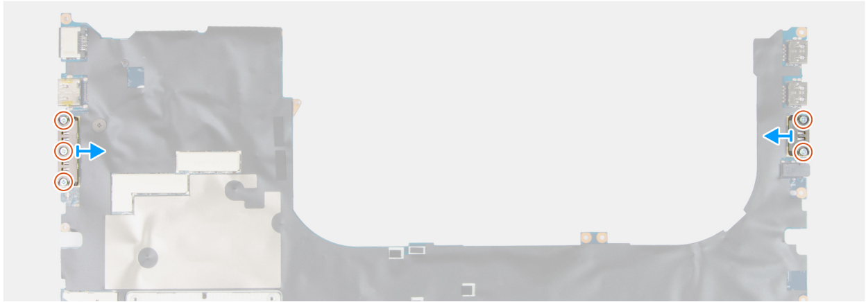
Figure 113. Removing the USB Type-C connector module
