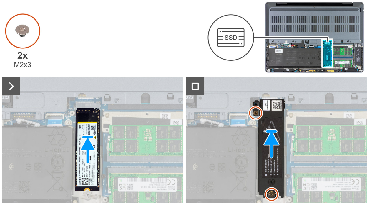
Figure 39. Installing the M.2 2280 SSD in slot 2 (SSD2)
