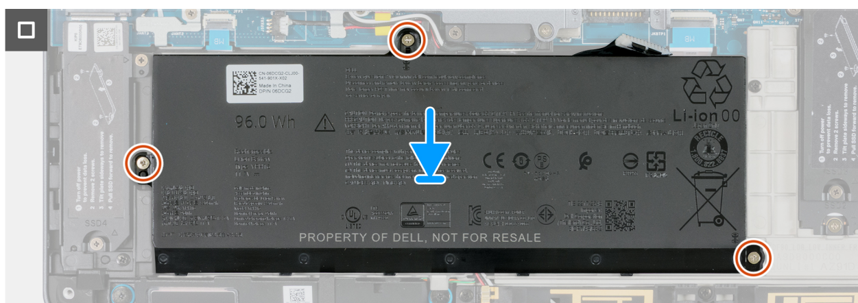
Figure 47. Replacing the battery
