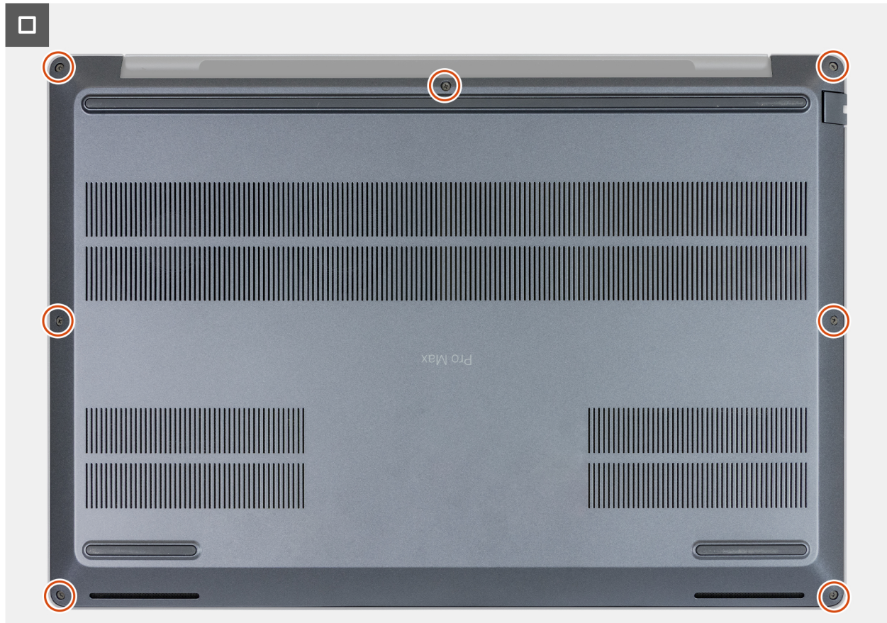
Figure 29. Tightening the captive screws
