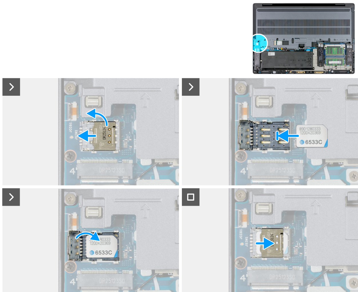
Figure 51. Installing the SIM card
