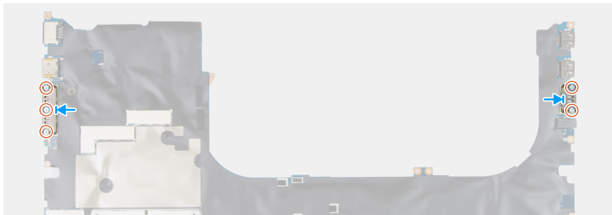
Figure 114. Installing the USB Type-C connector module
