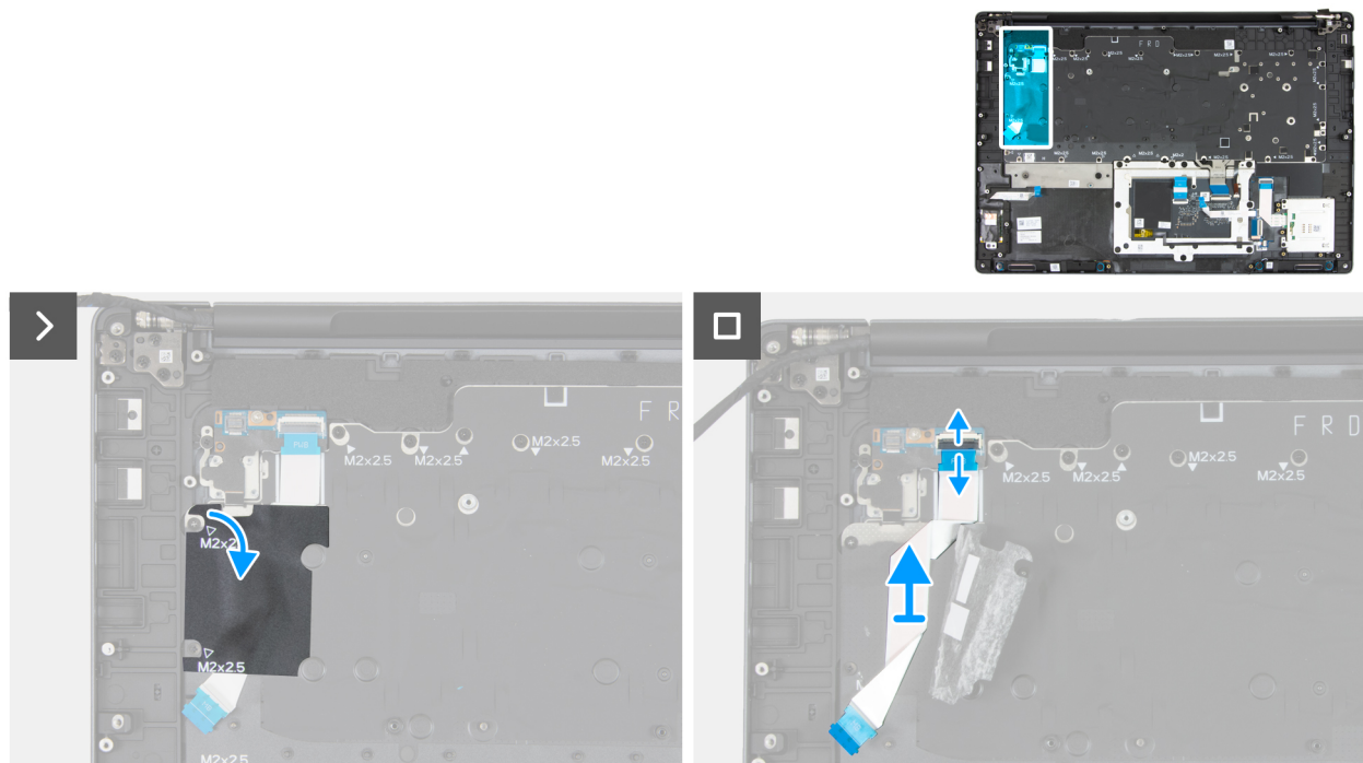
Figure 123. Removing the power button board cable
