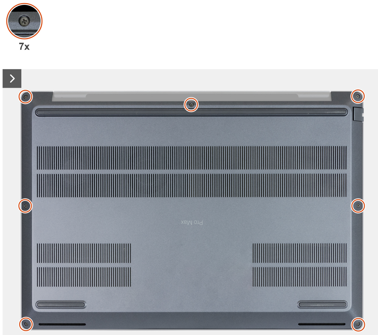
Figure 24. Loosening the captive screws
