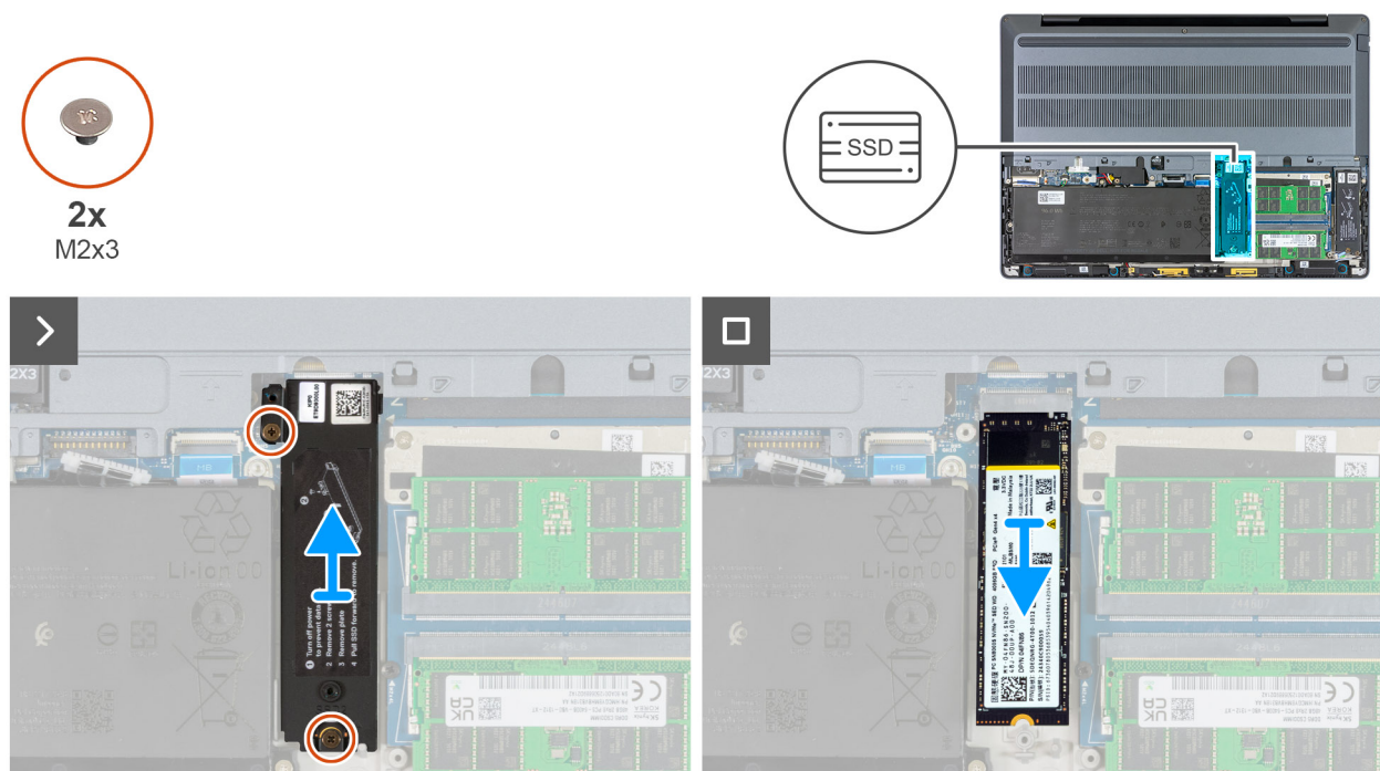
Figure 38. Removing the M.2 2280 SSD from slot 2 (SSD2)
