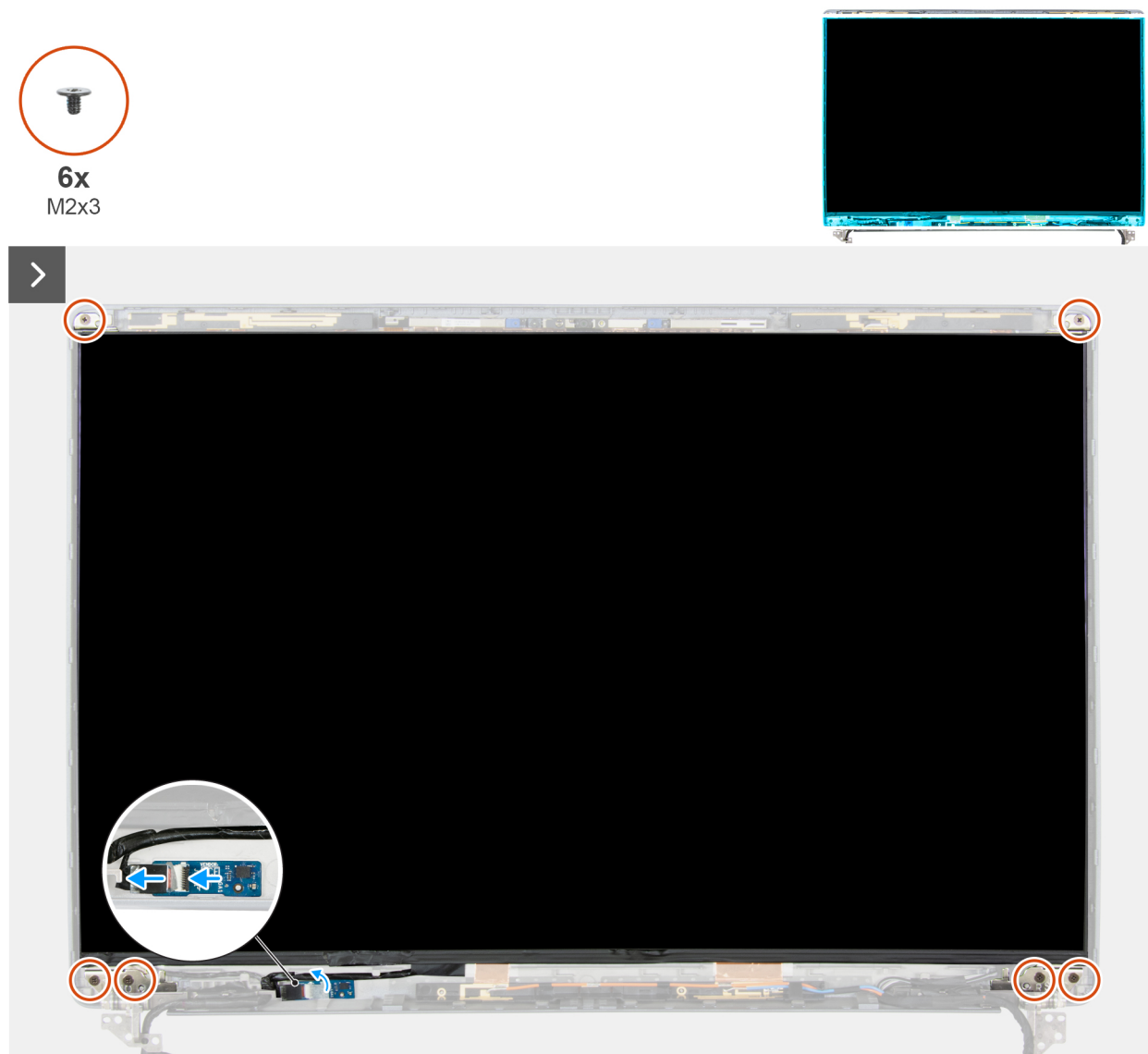
Figure 95. Removing the display panel
