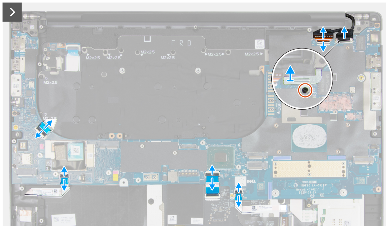
Figure 107. Removing the system board
