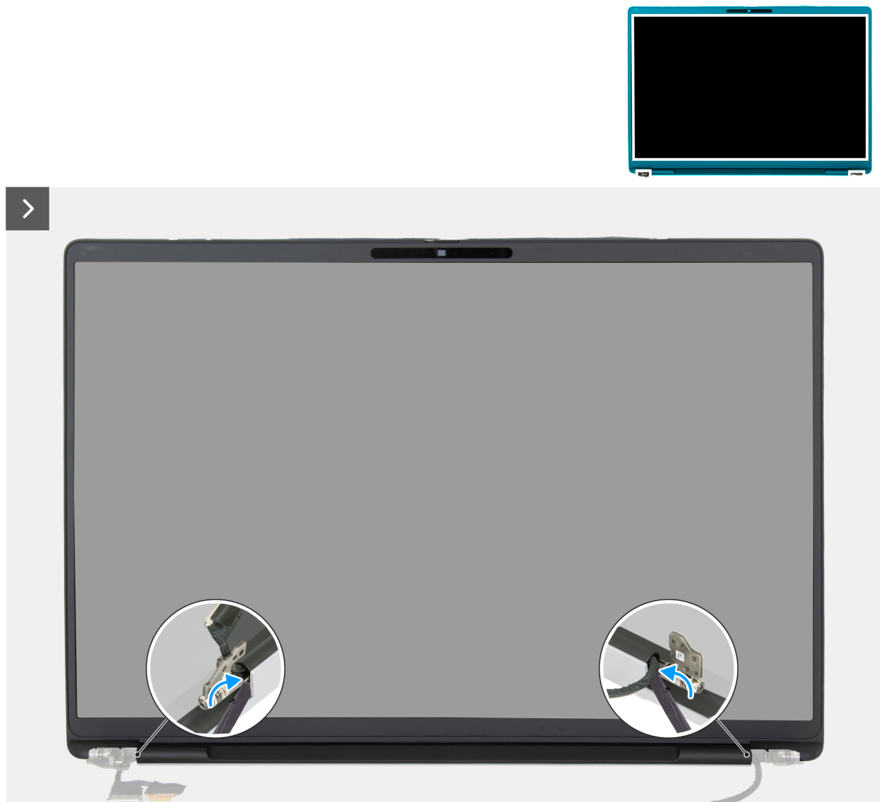
Figure 83. Removing the display bezel
