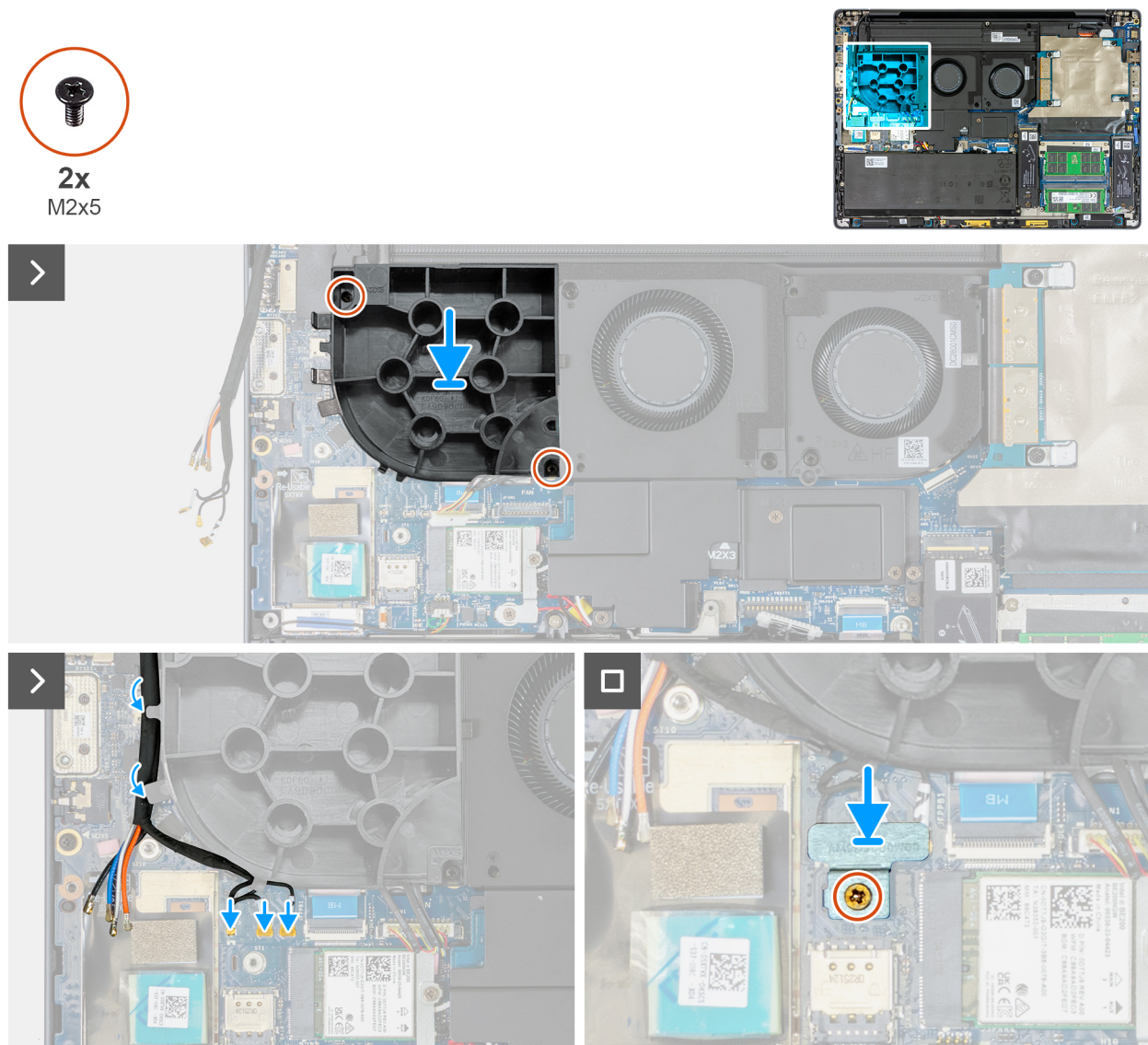
Figure 58. Installing the dummy fan
