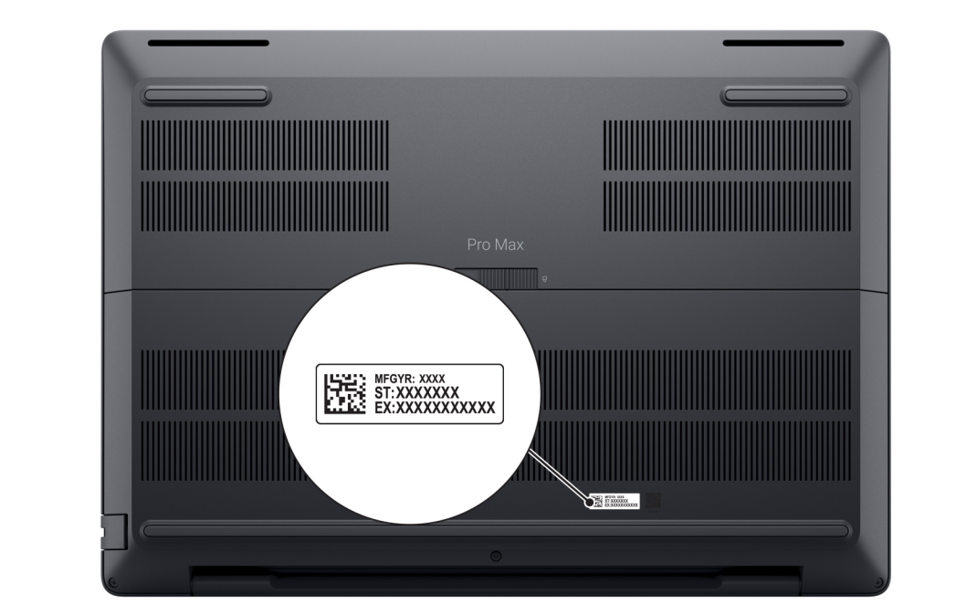
Figure 6. Service Tag/Express Service Code location
