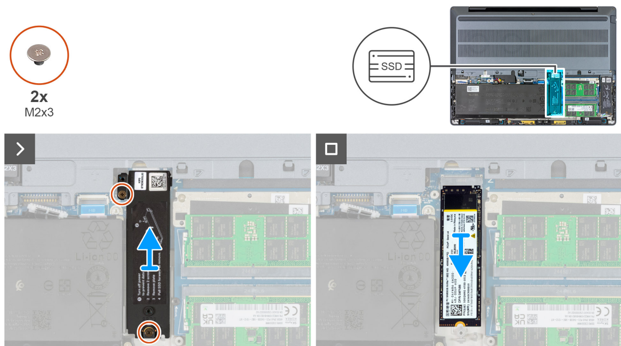
Figure 36. Removing the M.2 2280 SSD from slot 2 (SSD2)
