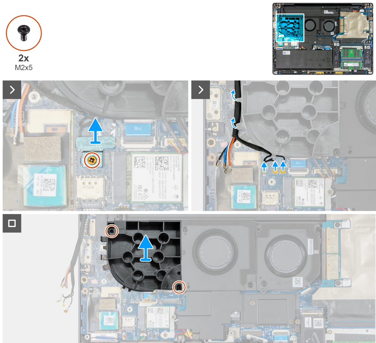
Figure 57. Removing the dummy fan
