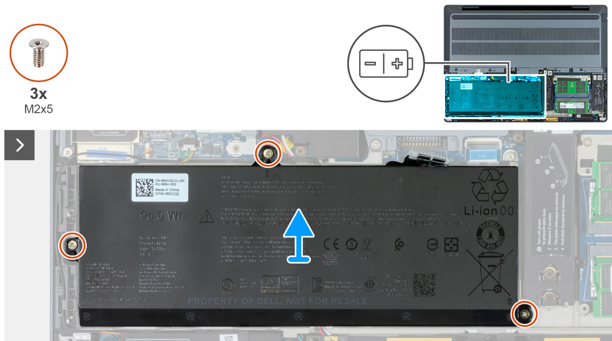
Figure 40. Removing the battery
