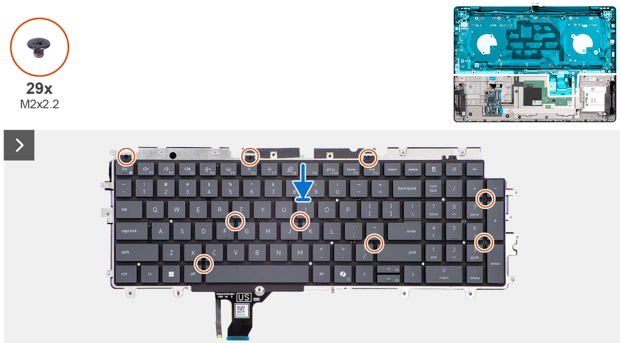
Figure 85. Installing the keyboard
