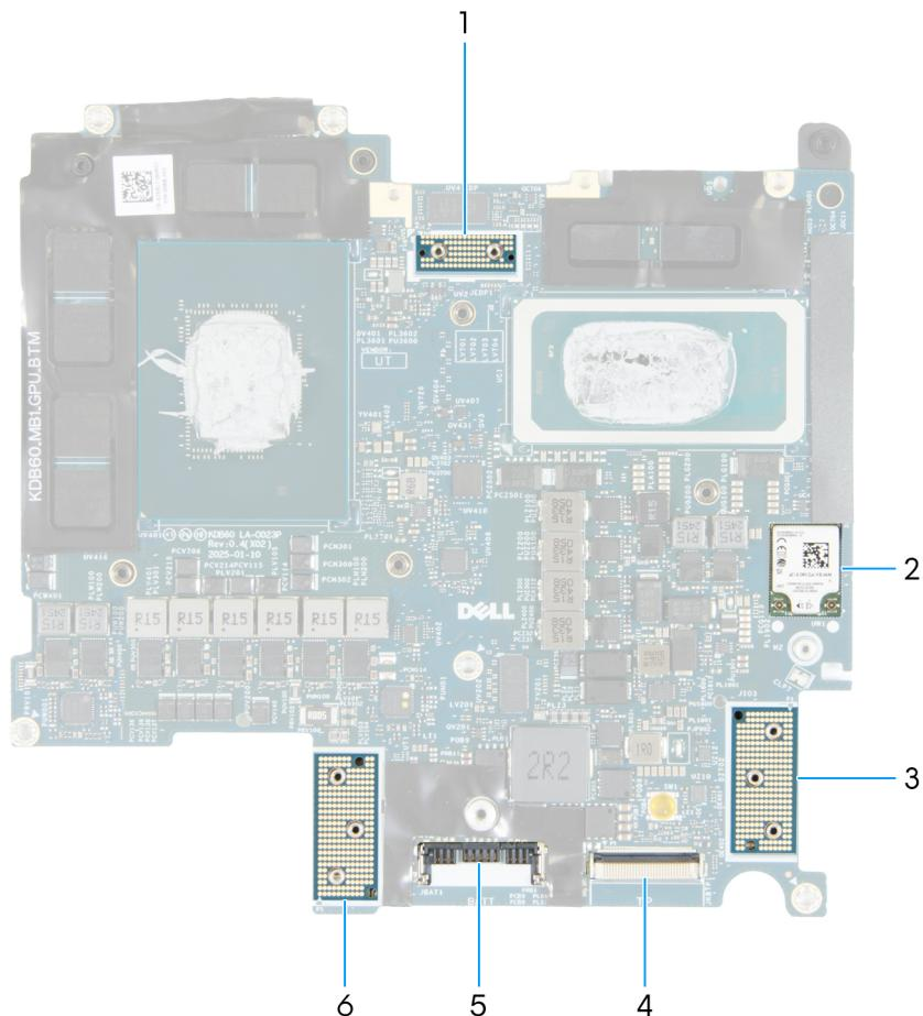
**Figure 63. System board connectors**
