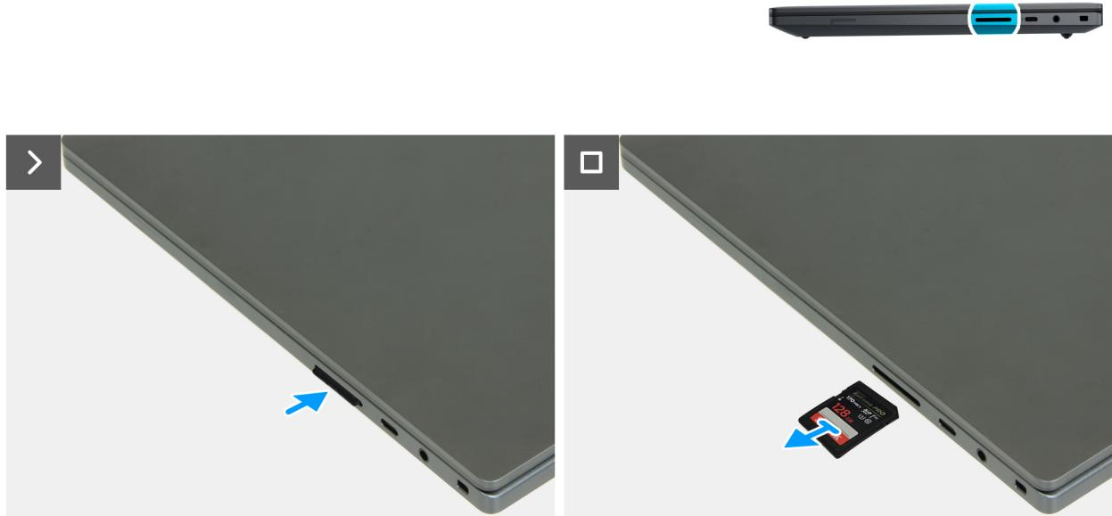
**Figure 11. Removing the memory card**
