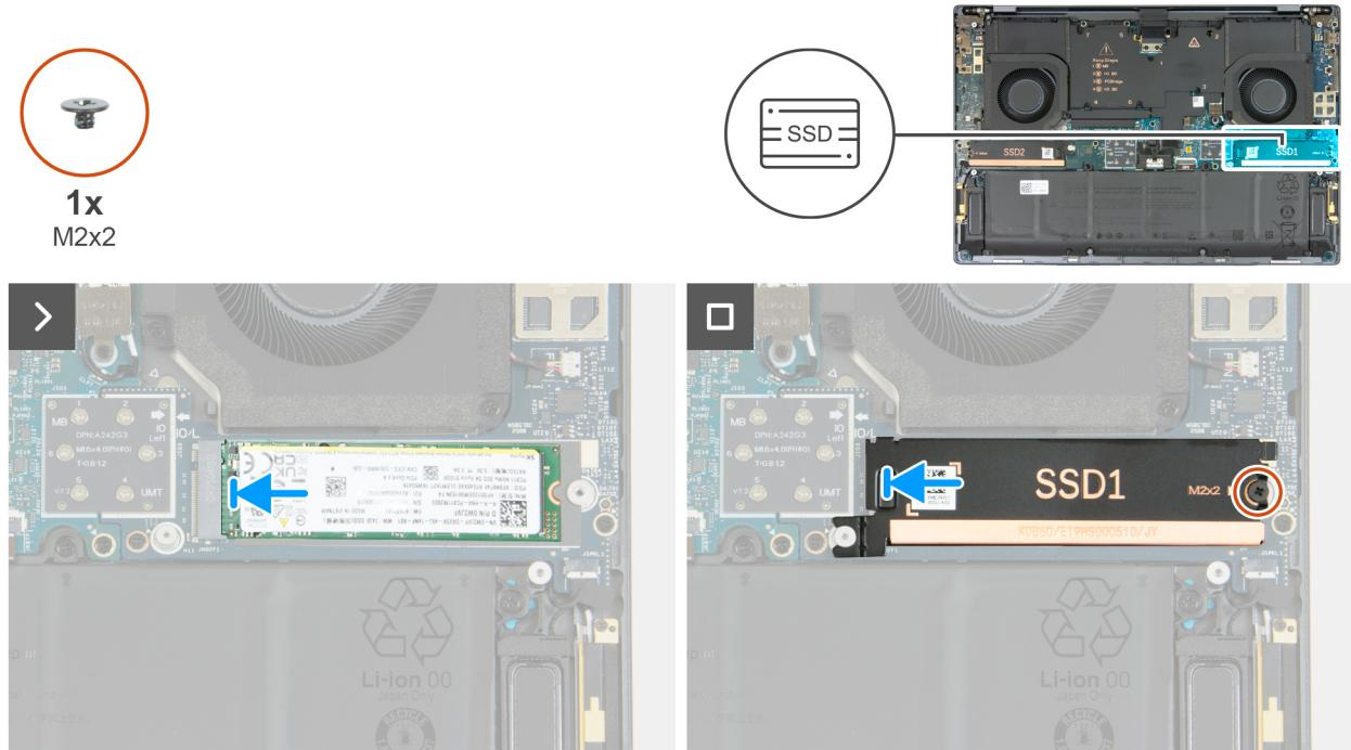
Figure 24. Installing the M.2 2280 solid state drive (SSD1)
