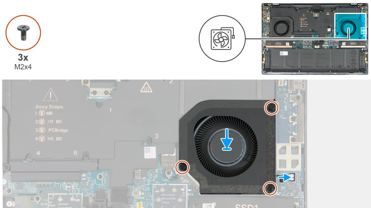
**Figure 31. Installing the left fan**
