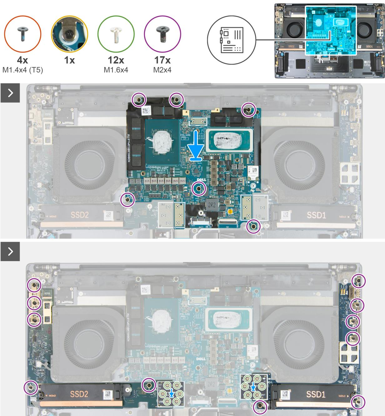
**Figure 68. Installing the system board (discrete graphics)**
