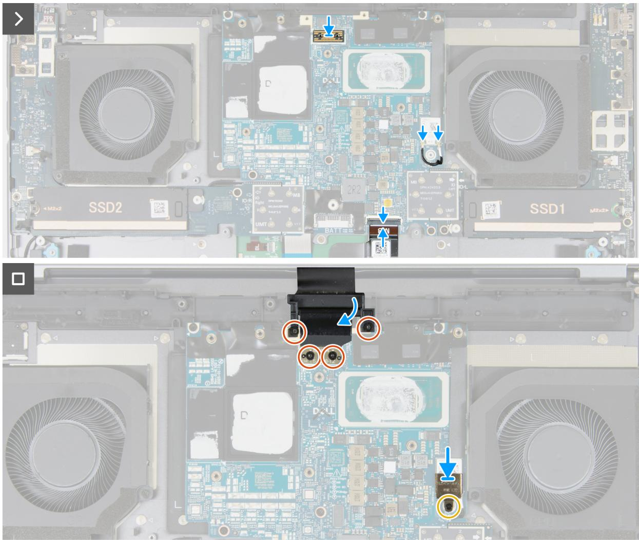
**Figure 60. Installing the system board (integrated graphics)**
