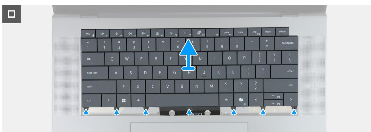
**Figure 77. Removing the keyboard**
