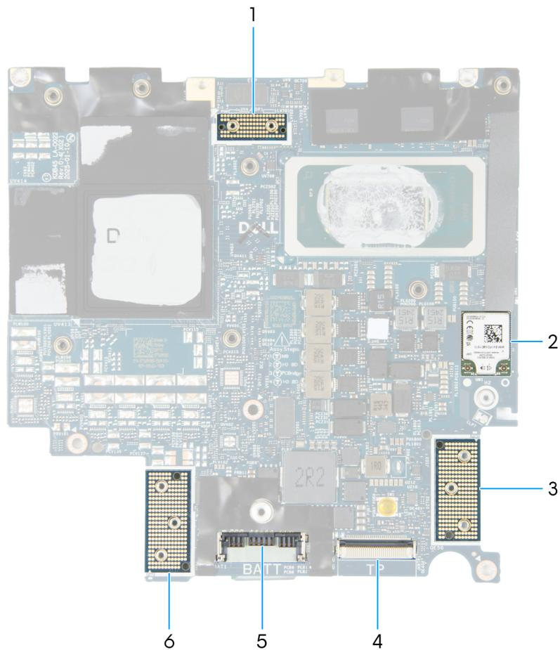
**Figure 58. System board connectors**
