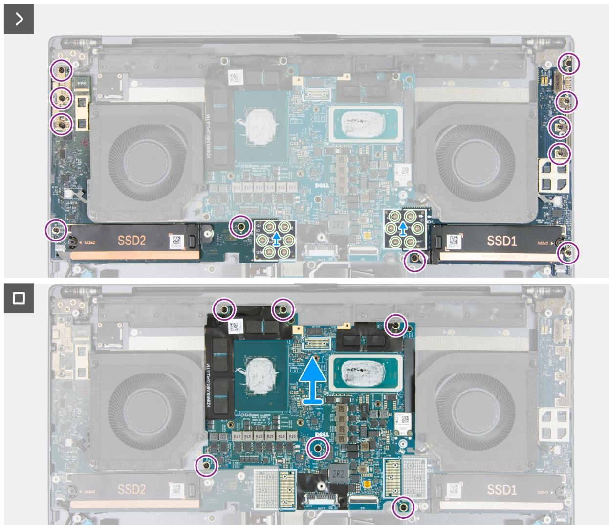
**Figure 65. Removing the system board (discrete graphics)**
