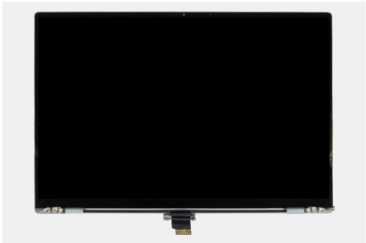
**Figure 41. Display assembly with touch screen**
