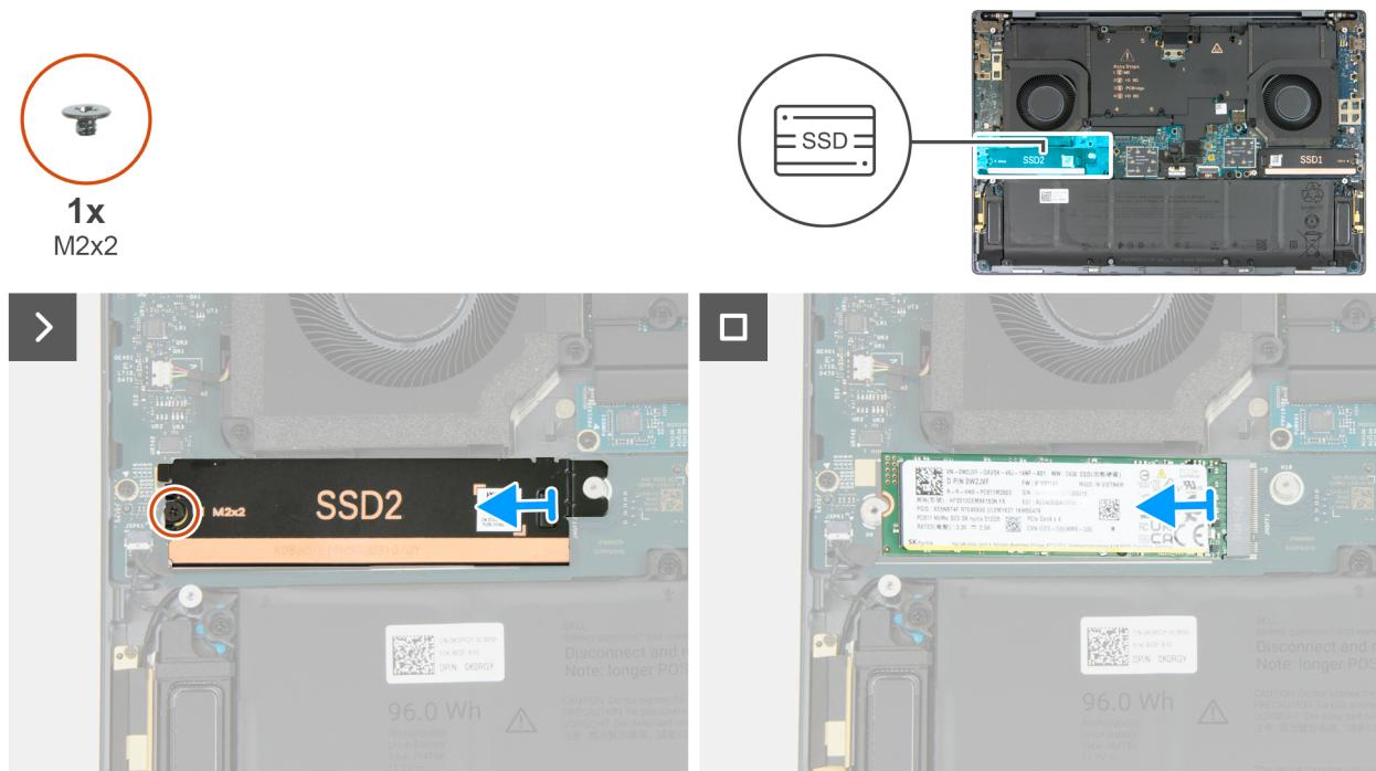
**Figure 23. Removing the M.2 2280 solid state drive (SSD2)**
