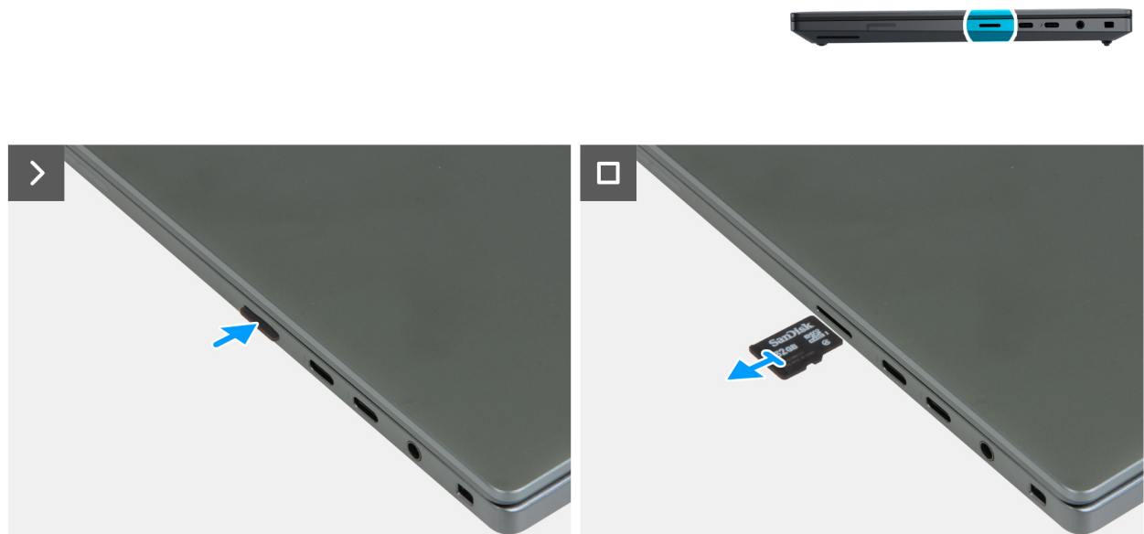
Figure 10. Removing the memory card
