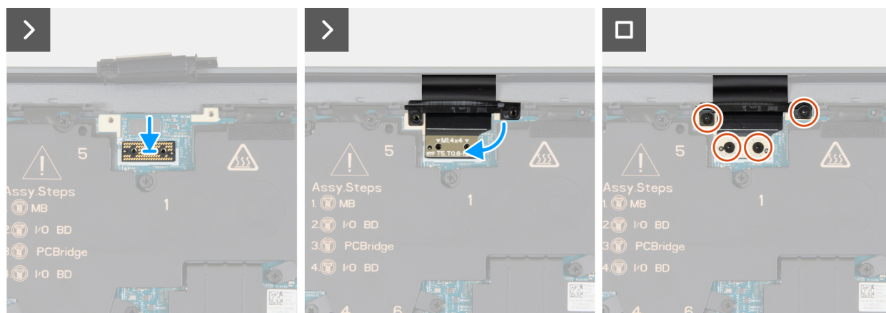
Figure 39. Installing the display assembly
