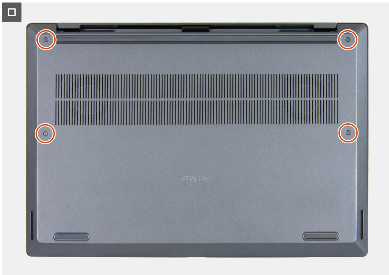
Figure 15. Installing the base cover
