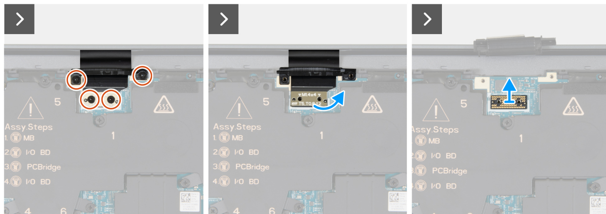
Figure 31. Removing the display assembly
