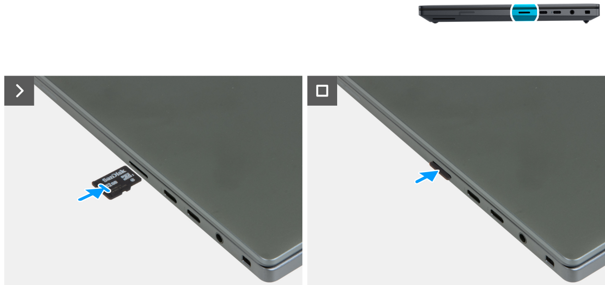
Figure 11. Installing the memory card
