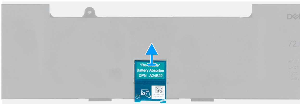
Figure 18. Removing the battery absorber
