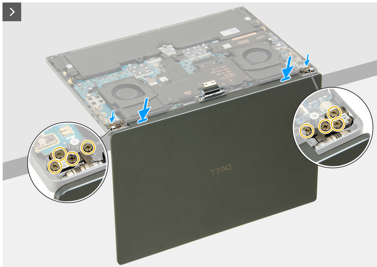
Figure 38. Installing the display assembly
