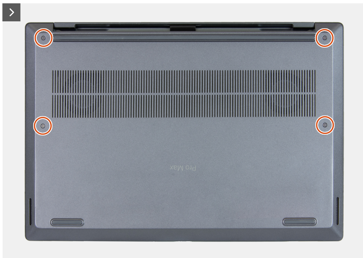
Figure 12. Removing the base cover
