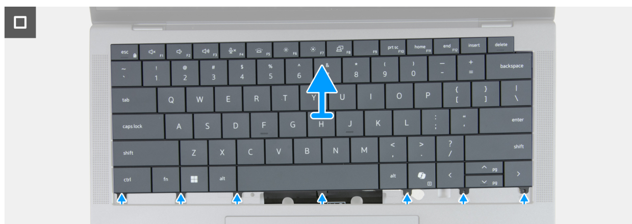
Figure 72. Removing the keyboard
