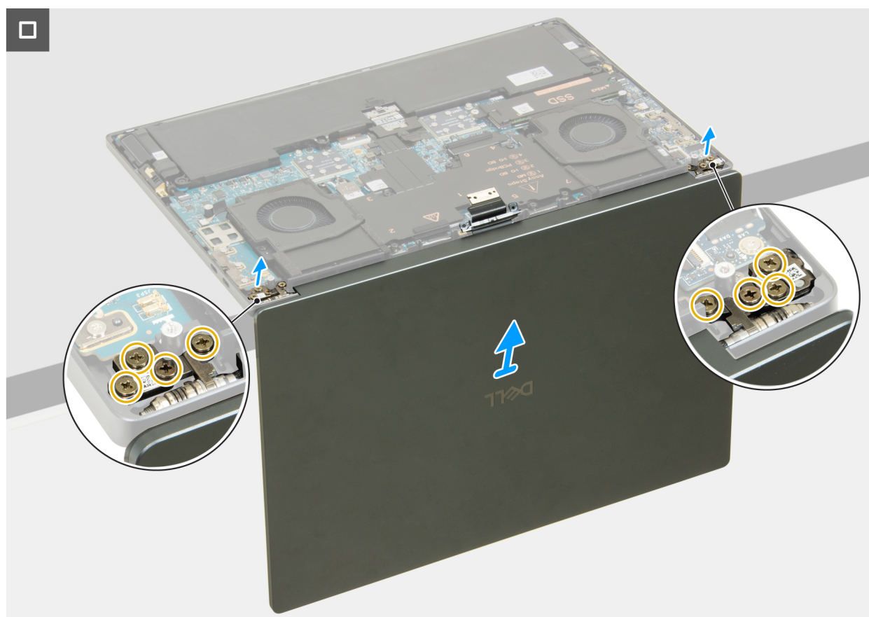
Figure 32. Removing the display assembly
