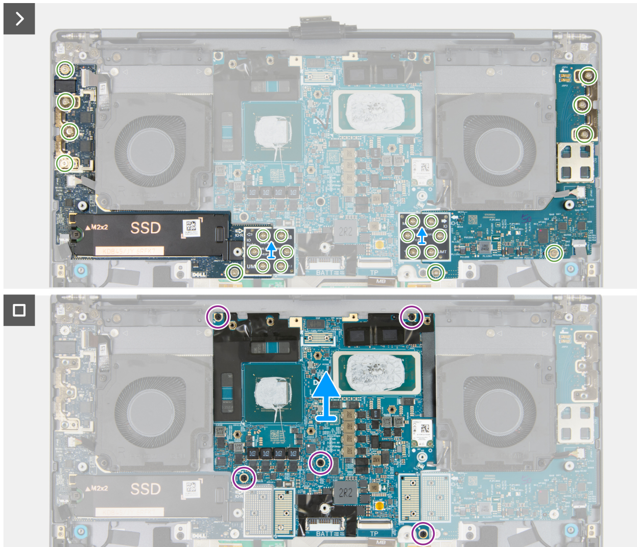
Figure 60. Removing the system board (discrete graphics)
