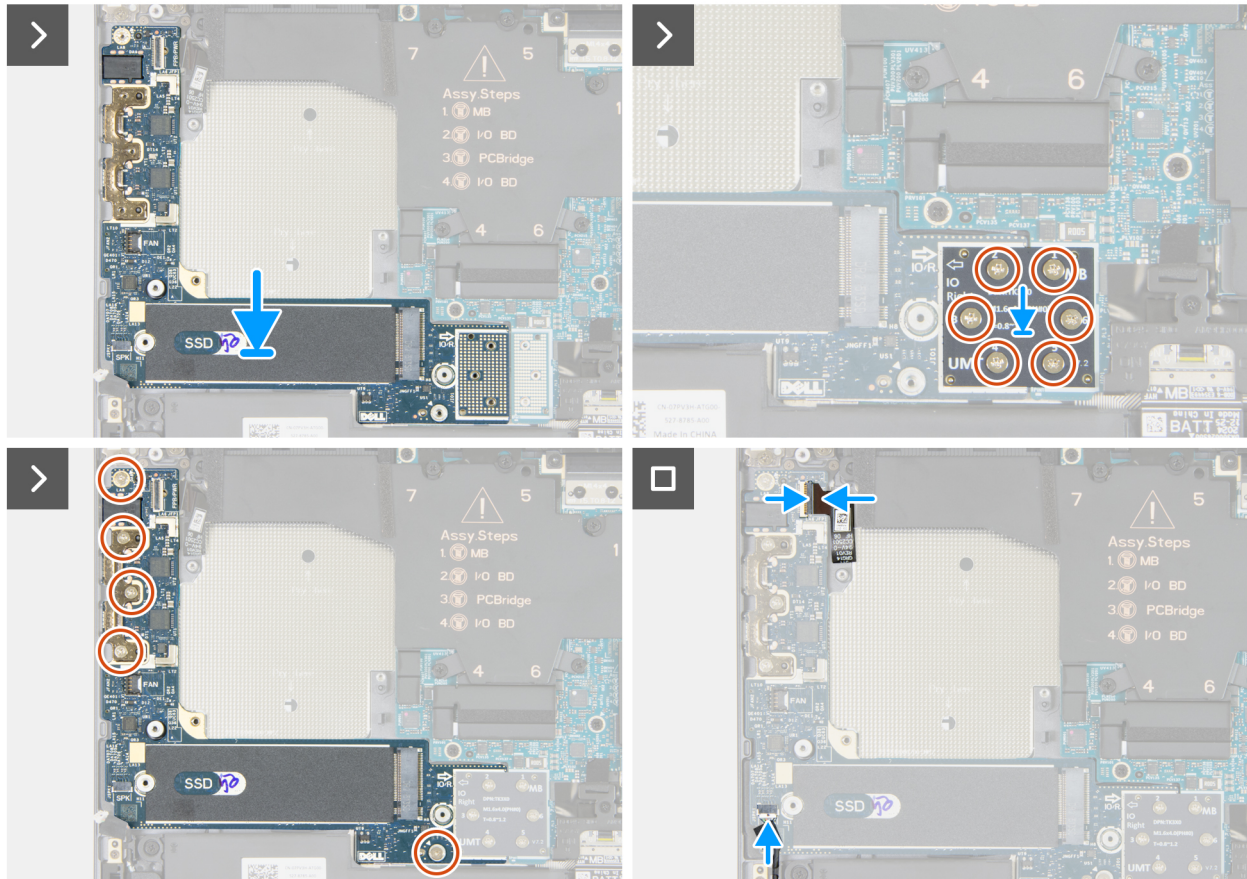
Figure 48. Installing the right I/O-board
