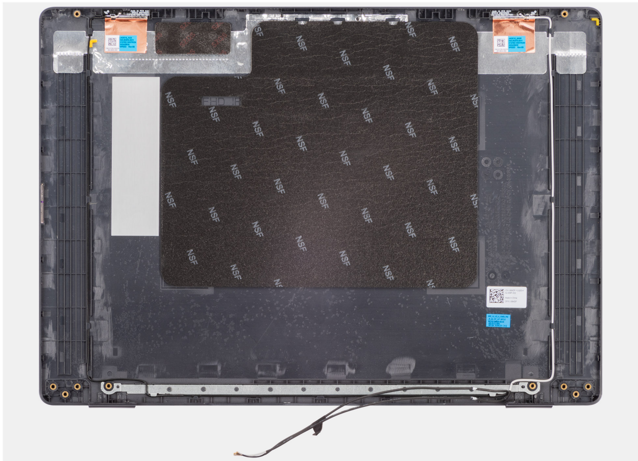
Figure 87. Installing the display back-cover assembly
