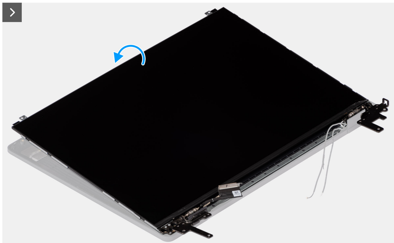
Figure 80. Installing the display-panel assembly
