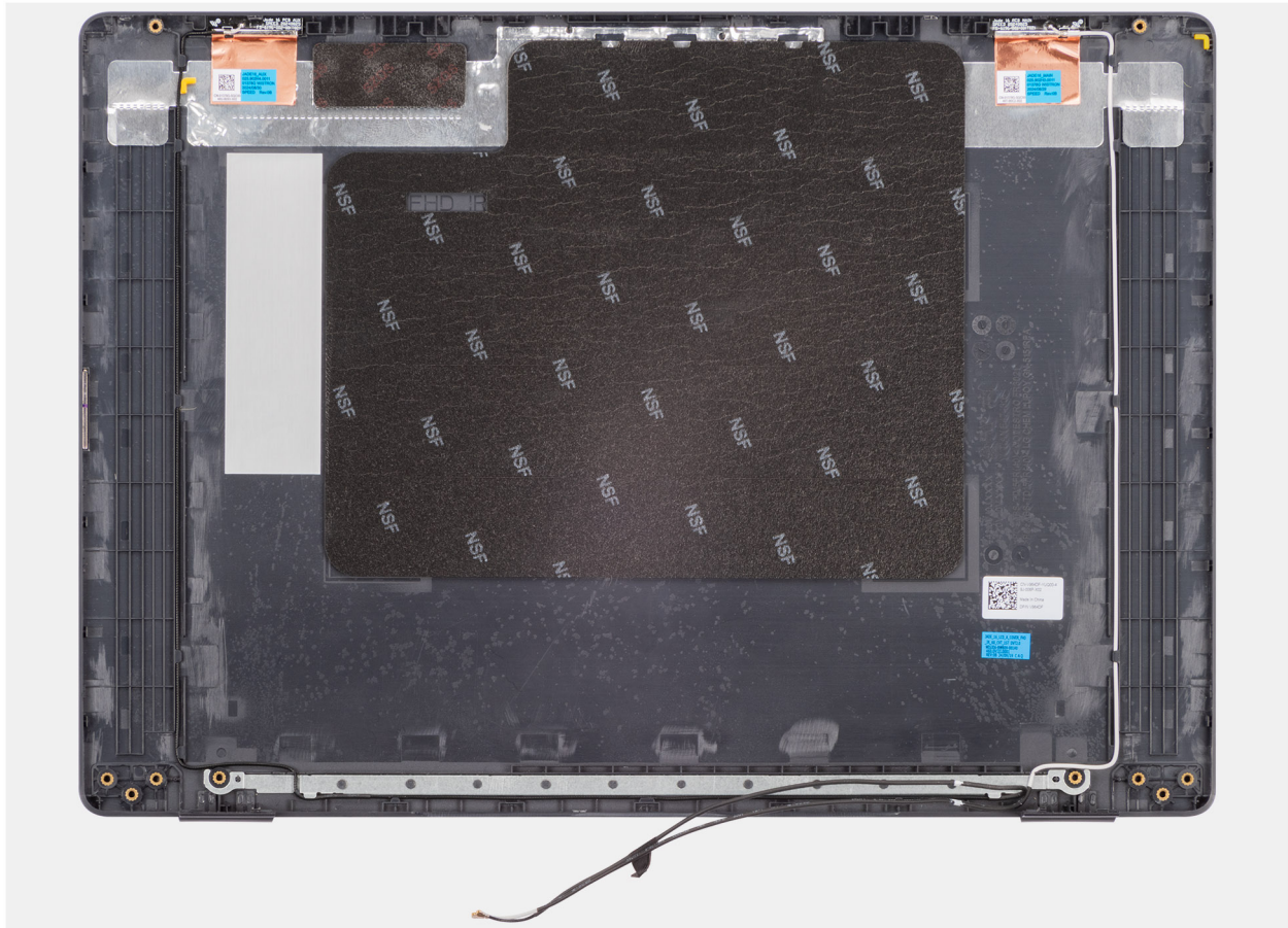
Figure 86. Removing the display back-cover assembly
