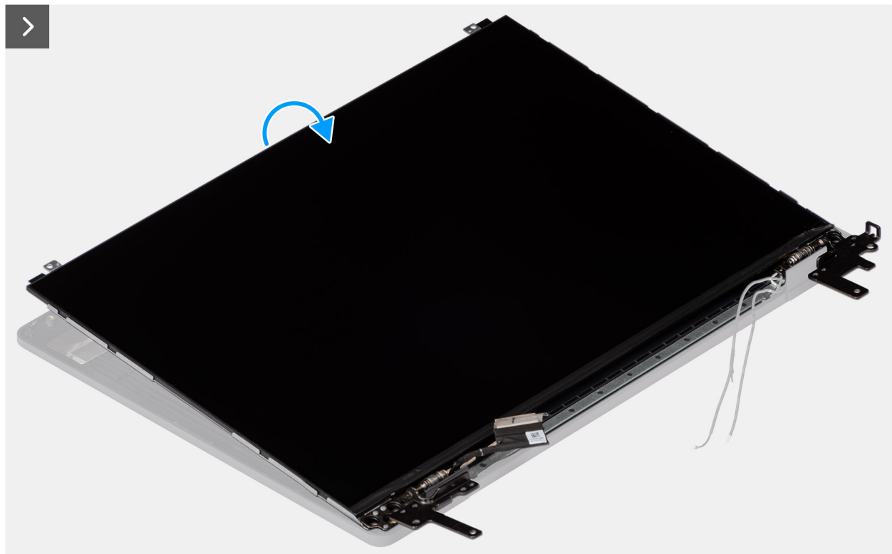
Figure 75. Removing the display-panel assembly
