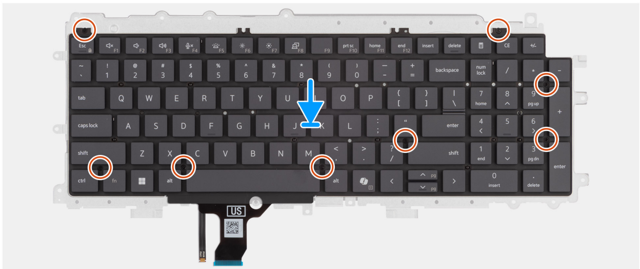
Figure 59. Installing the keyboard support plate
