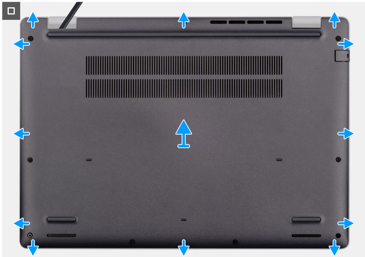
Figure 12. Removing the base cover
