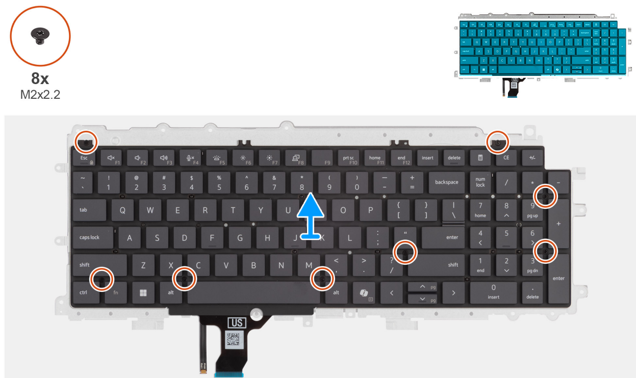
Figure 56. Removing the keyboard support plate
