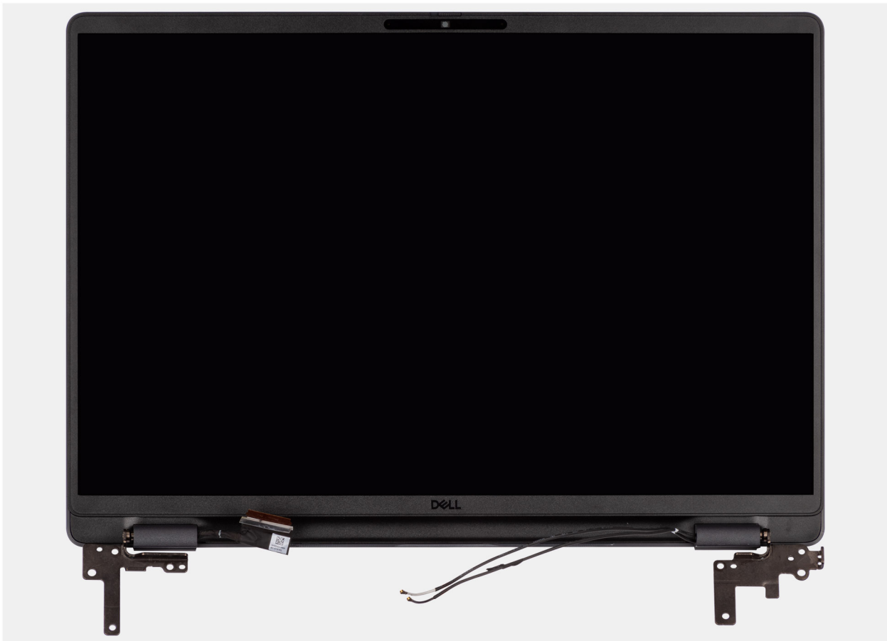
Figure 64. Removing the display assembly
