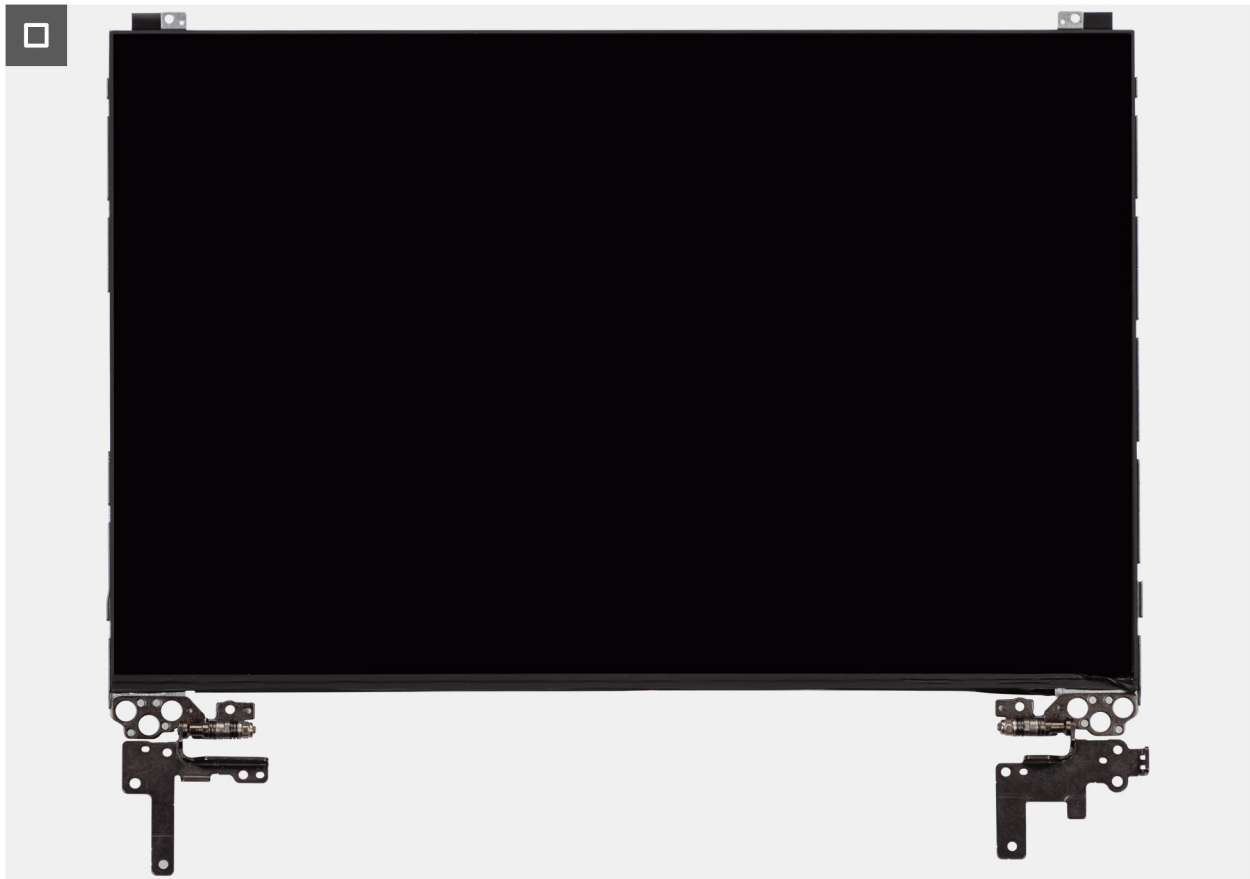
Figure 77. Removing the display-panel assembly
