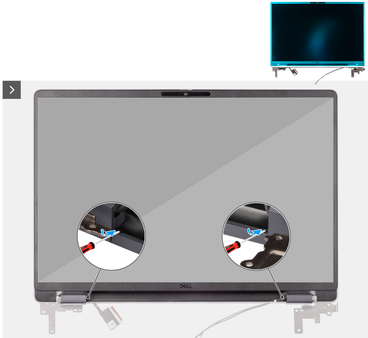
Figure 67. Removing the display bezel
