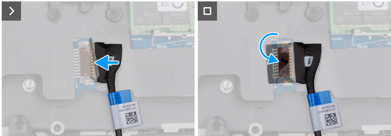
Figure 14. Connecting the battery cable
